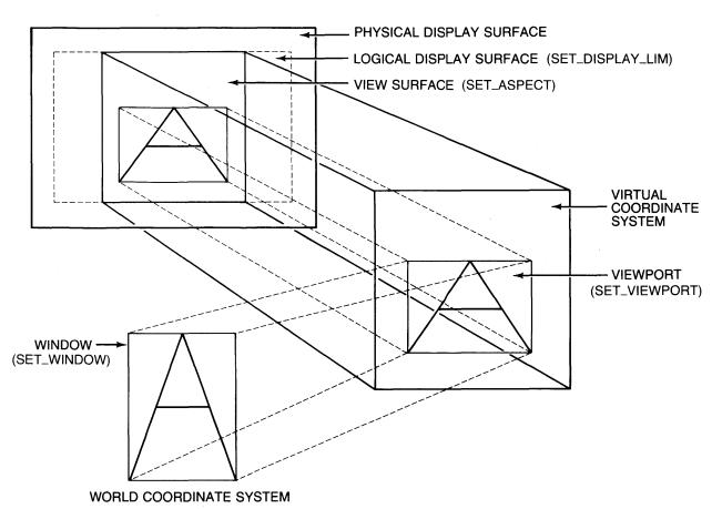
Quite often, a frame is desired around the current window to set it apart from the labels outside the window, and so forth. If the window limits are known (or it is convenient to find out), you can just do a MOVE and four LINEs, as was done in the last chapter. The way it was done in the last chapter was to draw the frame *after* the SET\_VIEWPORT call, but *before* the
