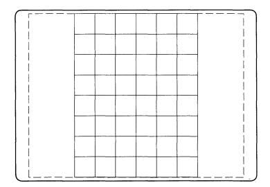
In the next example, the requested values were 0 to 7 in X, and 0 to 4 in Y. Since the aspect ratio of this window is greater than the aspect ratio of the viewport, some extra room is needed in the Y direction, as shown.
