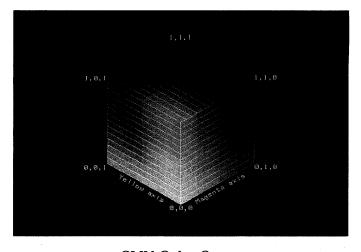
CMY Color Space NOTE: This photo is a multiple exposure of Model 236 Color Computer CRT.
