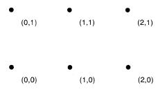
1 The word "pixel" is a blend of the two words "picture element," and it is the smallest addressable point on a plotting surface. A Model 236 computer has 512 × 390-pixel resolution; thus there can be no more than 512 dots drawn in any one row of the CRT, or 390 dots drawn in any one column.
