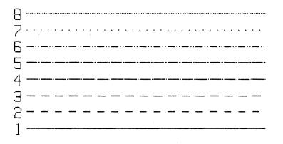
As you can see, line style 1 draws a solid line. Line styles 2 through 8 are patterned sequences of on and off. For all line styles, the computer remembers where in the pattern a line segment ended. Therefore, when you start drawing another line segment, the line pattern will continue from where it left off. If you want the pattern to start over, just re-execute the line style procedure.
