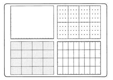
Note that some care must be taken to ensure that the minor tick marks in a grid are smaller than the distance between them. If they are not, the minor tick crosses drawn by the grid procedure would have overlapped. The end result would have been a grid with even the minor ticks extending all the way across the soft clip area.
