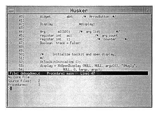
Figure 10-5. Running debugdemo With cdb
