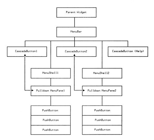
Figure 6-13. Creating a Pulldown Menu System Without Using Convenience Functions
