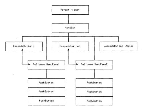
Figure 6-9. Creating a Pulldown Menu System With Convenience Functions
