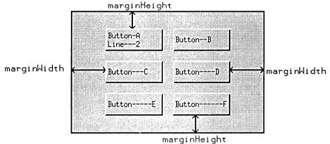
Figure 7-12. XmNmarginHeight and XmNmarginWidth
