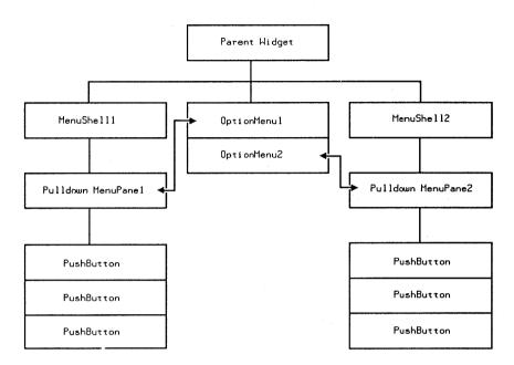
Figure 6-15. Creating an Option Menu System Without Using Convenience Functions
