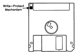
Figure 2-1: Flexible Disc Write Protect Mechanism
