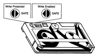
Figure 2-13: Tape Write Protect Mechanism
