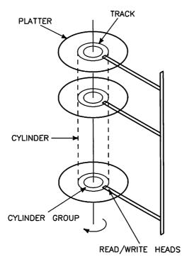
Figure G.1: Track, Cylinder, and Cylinder Group on a Disc
