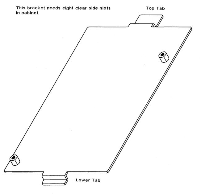
figure 2-8 option 550 mounting bracket for rs-232 connection box
