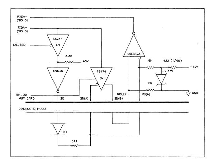
Figure 3-7. Diagnostic Test Hood Schematic Diagram
