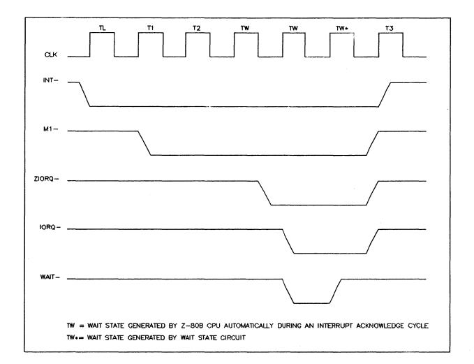
Figure 3-6. Wait State Circuit Timing Diagram
