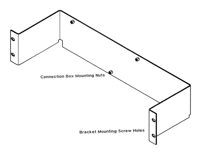
Figure 2-6. Option 019 Mounting Bracket for RS-232 Panel
