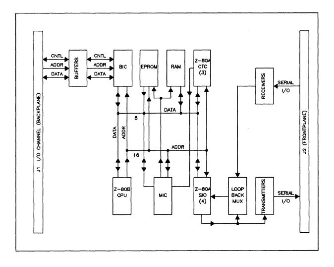
Figure 3-1. MUX Functional Block Diagram
