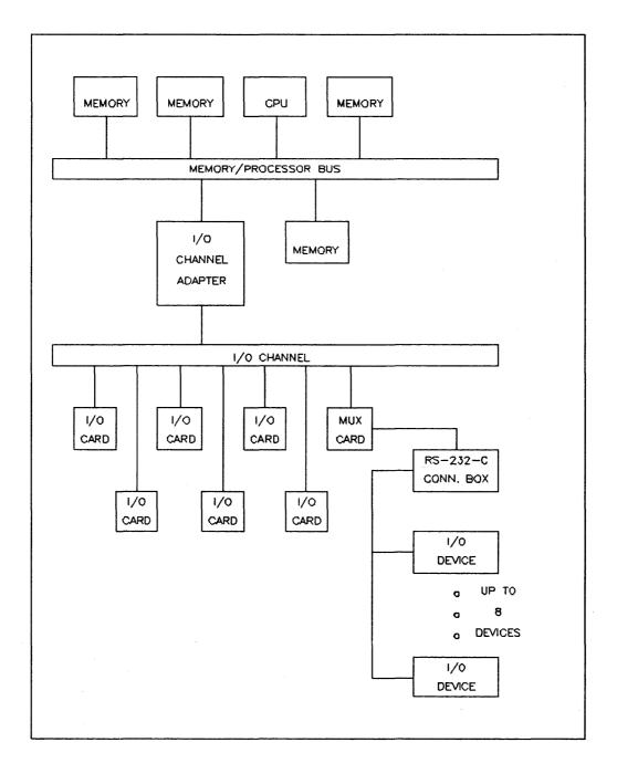
Figure 1-1. MUX In a Typical Hewlett-Packard Computer System
