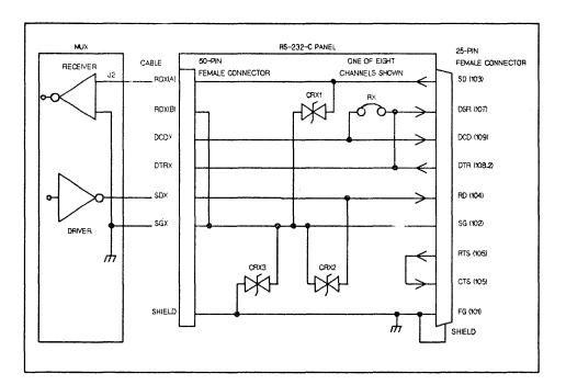
Figure 2-4. Connections From MUX-to-Panel-to-Device
