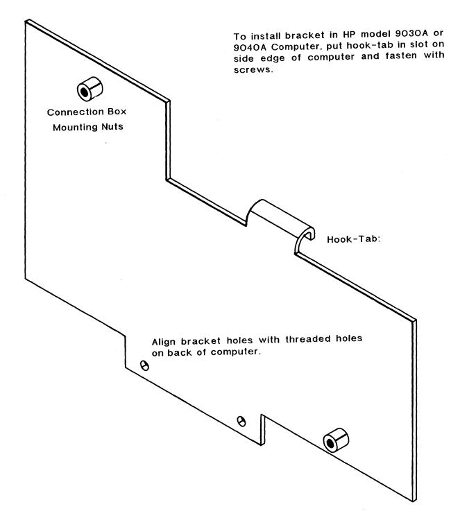
Figure 2-7. Option 540 Mounting Bracket for RS-232C Panel
