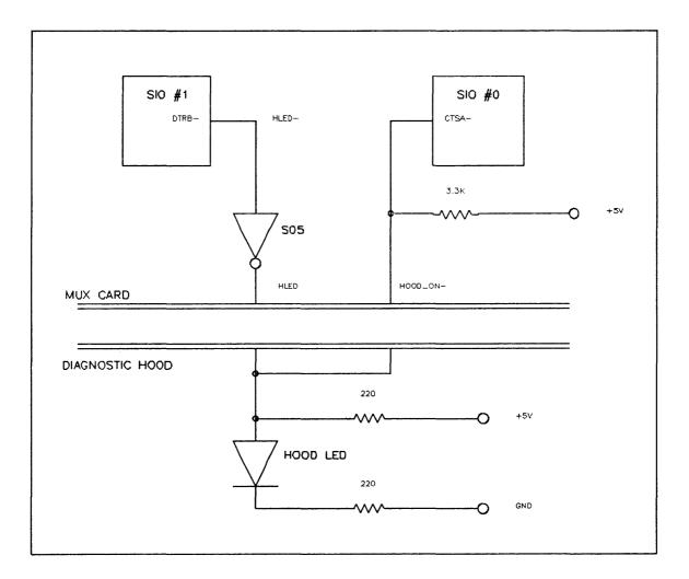
Figure 3-4. Diagnostic Hood LED Control Circuit and Hood Sense Circuit
