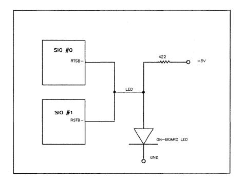
Figure 3-3. Control Circuit for the MUX Card LED
