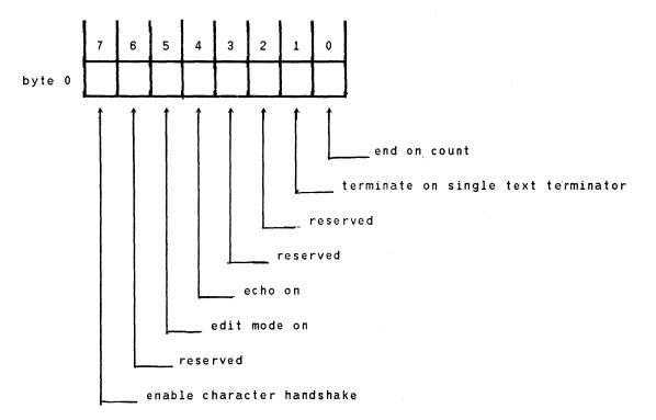
Validation : If the echo bit is set, the transmission mode must be full duplex. The transmission mode must be programmed first before setting the read option.
