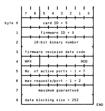
MPX = 1 for in-channel multiplexingMOD = 2 for both byte and word mode data transfers
