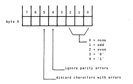
Validation : The value of bits 0-2 must be within the range 0 through 4, inclusive.
