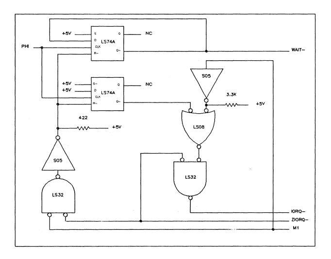
Figure 3-5. Wait State Circuit Schematic Diagram
