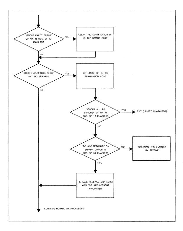
FIGURE 4-2. ERROR HANDLING FLOW CHART
