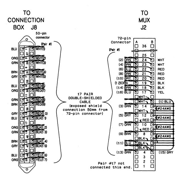
Figure 2-5. MUX to RS-232C Panel Cable
