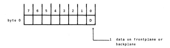
Subfunction 250. Get Card RAM. The uppermost 16K bytes of card RAM memory is sent to the host in the data block. (The other 32K bytes of RAM are not used by the MUX firmware.) The host buffer must be large enough to hold the data.
