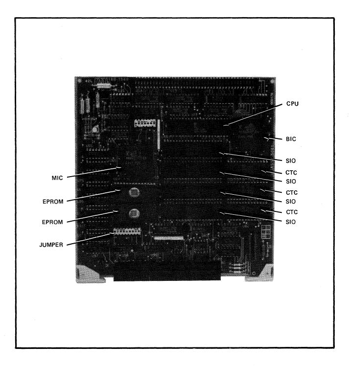
Figure 2-1. Component and Jumper Locations
