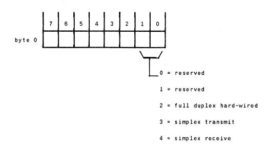
Validation : The parameter value must be within the range 2 through 4, inclusive. The transmission mode must be set before setting the read option. Note that the echo bit will be reset if the transmission mode is not full duplex.
