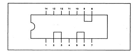
Figure 2-3. Signature Analysis Jumper Internal Connections
