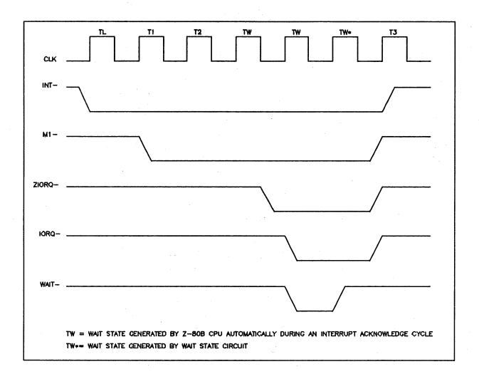
Figure 3-6. Wait State Circuit Timing Diagram
