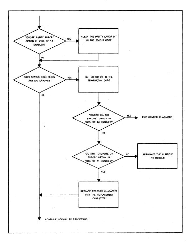
Figure 4-2. Error Handling Flow Chart
