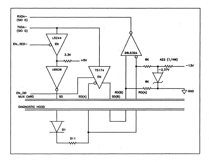
Figure 3-7. Diagnostic Test Hood Schematic Diagram
