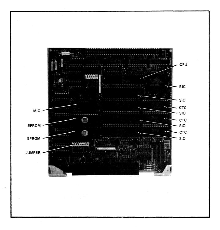
Figure 2-1. Component and Jumper Locations
