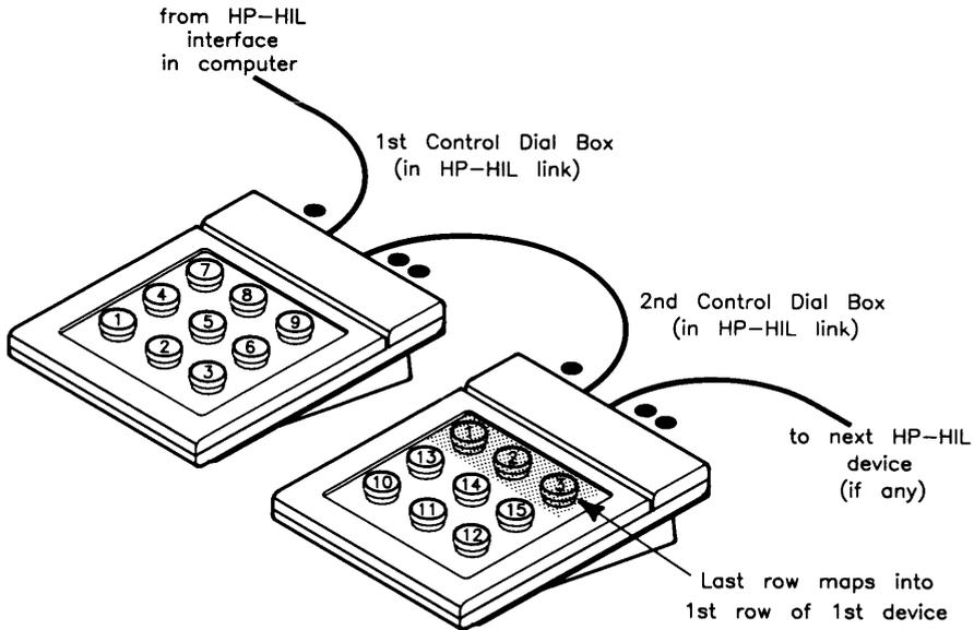
Once CDIAL is used to read information about a particular dial (registers 1 thru 15), that register is automatically cleared as is the corresponding bit in register 0. Reading register 0 does not change register 0.
