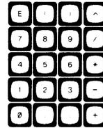
The numeric keypad provides a convenient way to enter numbers and perform arithmetic operations. Simply type in the arithmetic expression you want to evaluate, then press **EXECUTE**. The result is displayed in the lower-left corner of the screen.
