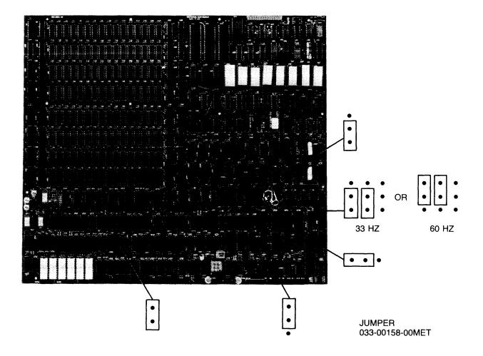
Figure 1-1. Controller Pc Assembly Jumpers
