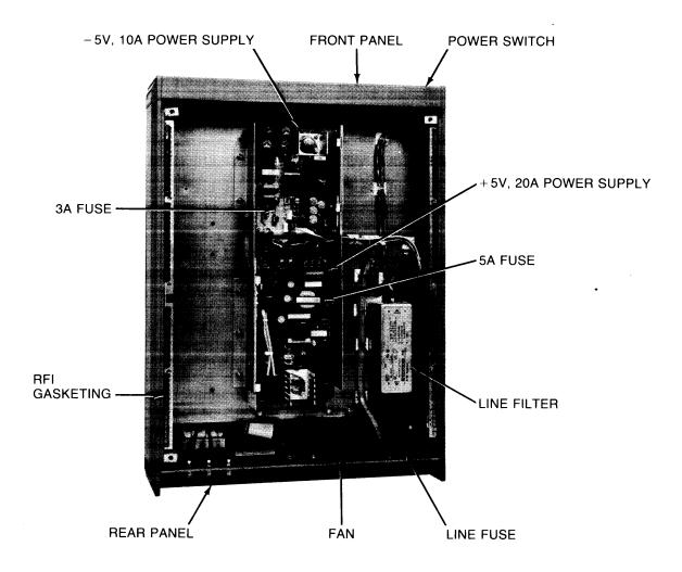
Figure 5-2. Replaceable Parts, Bottom View
