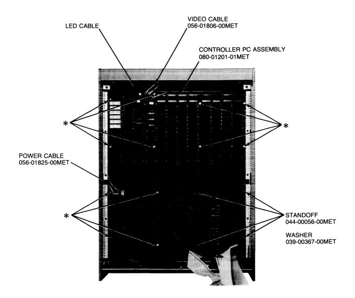
\* SCREW 038-01473-00MET SLEEVE OVER STANDOFFS UNDER CONTROLLER PC ASSEMBLY 044-01745-00MET
