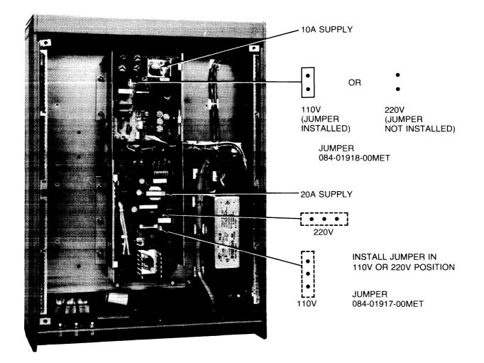
Figure 1-4. Power Supply Voltage Jumpers
