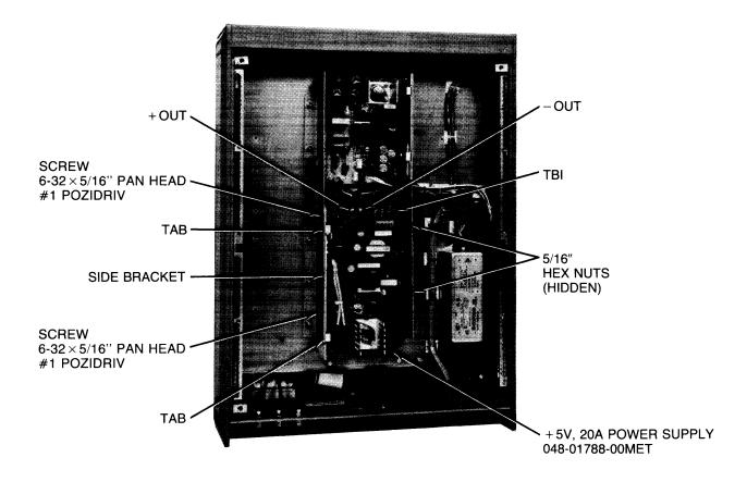
Figure 4-7. + 5V, 20A Power Supply
