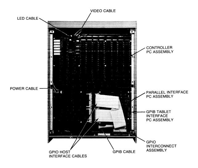
Figure 5-1. Replaceable Parts, Top View
