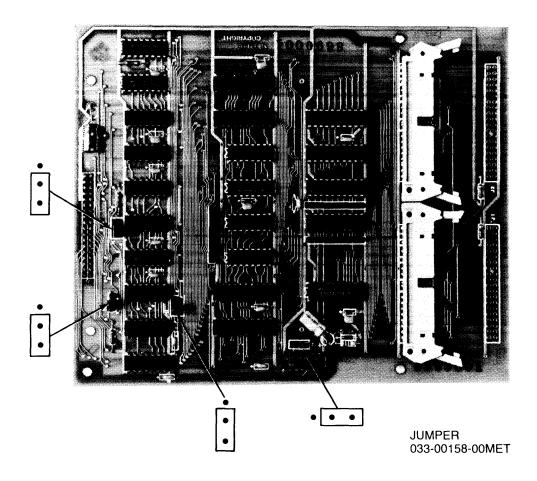
Figure 1-2. Parallel Interface Pc Assembly Jumpers
