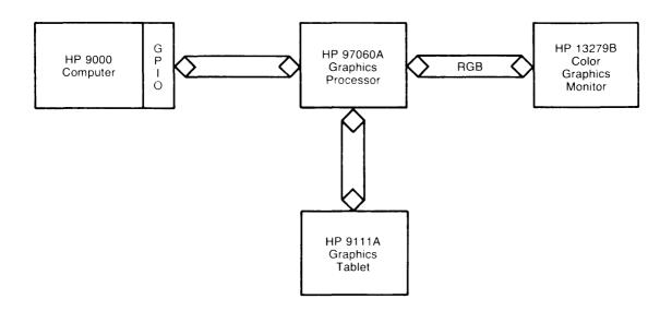
Figure 2-1. System Block Diagram
