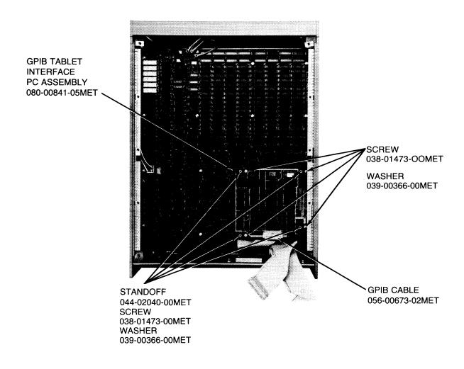
Figure 4-4. GPIB Tablet Interface Pc Assembly
