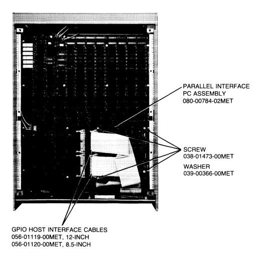
Figure 4-3. Parallel Interface Pc Assembly
