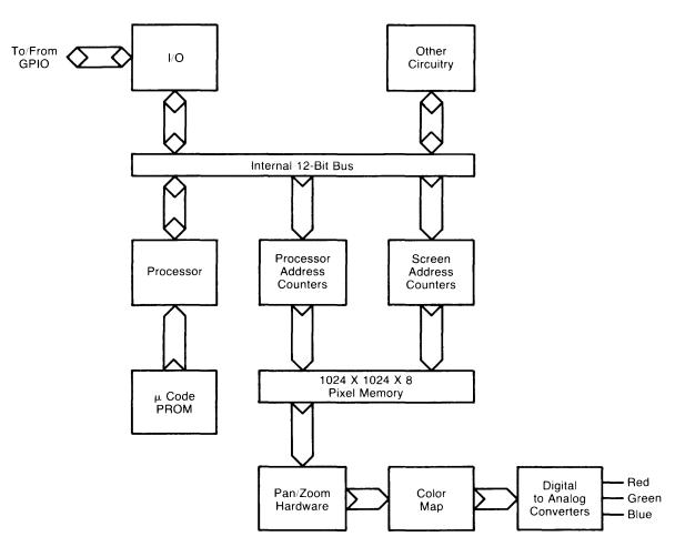
Figure 2-2. 97060A Block Diagram
