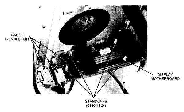
Figure 4-85. Removing Display Motherboard
