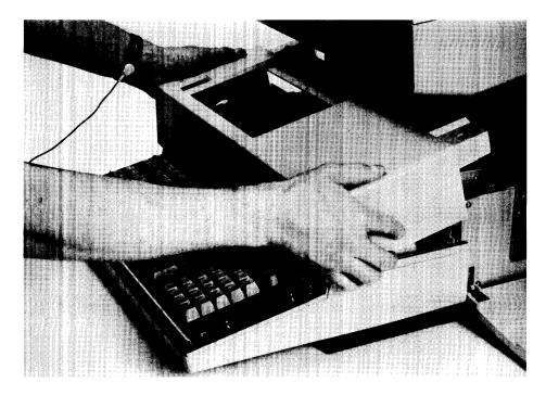
6. Lift rear of front cover and slide cover forward and away from computer (Figure 4-6).
