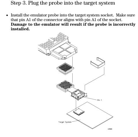
You can also use the supplied PGA to PGA adapter or other PQFP adapters. Always make sure that pin 1 and other pins of the adapters and connectors are properly aligned; otherwise, damage to the emulator will result.
