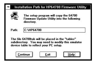
Chapter 15: Installing/Updating HP 64700 Firmware Step 2. Install the firmware update utility
