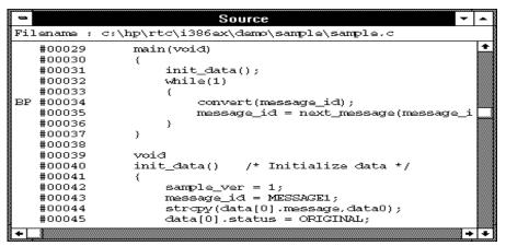
Notice that line 34 is marked with "BP", which indicates a breakpoint has been set on the line.
