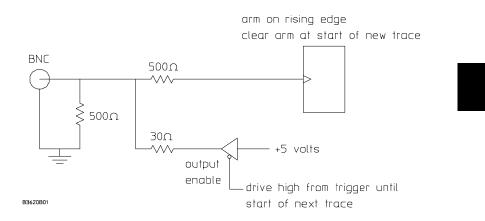
When a trace starts, it stops driving the output (so if nothing else is driving the line, it will fall low due to the 500 ohm pull-down resistor).
