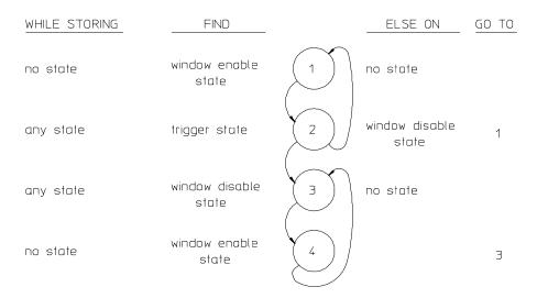
Notice that the order of the second sequence level pair is swapped. In sequence level 2, if the analyzer finds the trigger condition while searching for the window disable state, it will branch to sequence level 3 where it continues its search for the window disable state. After this, the analyzer will remain in sequence levels 3 and 4 until the trace memory is filled, completing the trace.
