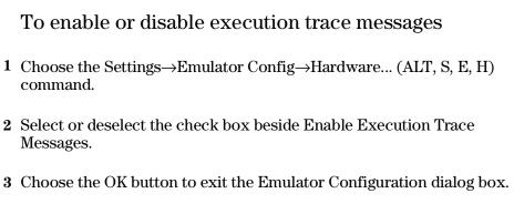
When the check box is selected, branch trace messages and task switch messages are enabled. Every time the processor does a branch, it will emit the target address of the branch. Each time a task switch occurs, the emulator will emit a task switch message identifying both the old task and the new task.
