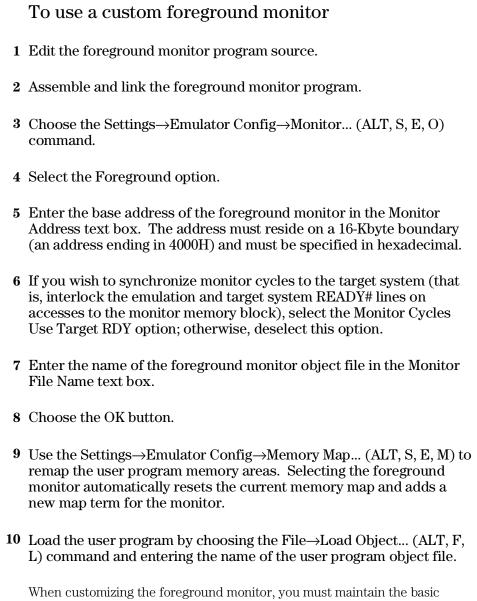
When customizing the foreground monitor, you must maintain the basic communication protocol between the monitor program and the emulation system controller.
