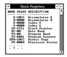
The Register window opens and displays the register contents. The display is updated periodically. To run the program and see how the contents of the registers change:
