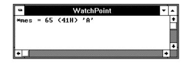
The contents of dynamic variables are displayed only when the current program counter is in the function in which the variable is declared.
