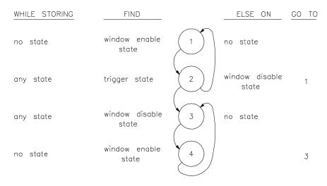
Notice that the order of the second sequence level pair is swapped; if you find the trigger condition while searching for the window disable state, you want the analyzer to branch to a sequence level that continues to search for the disable state.
