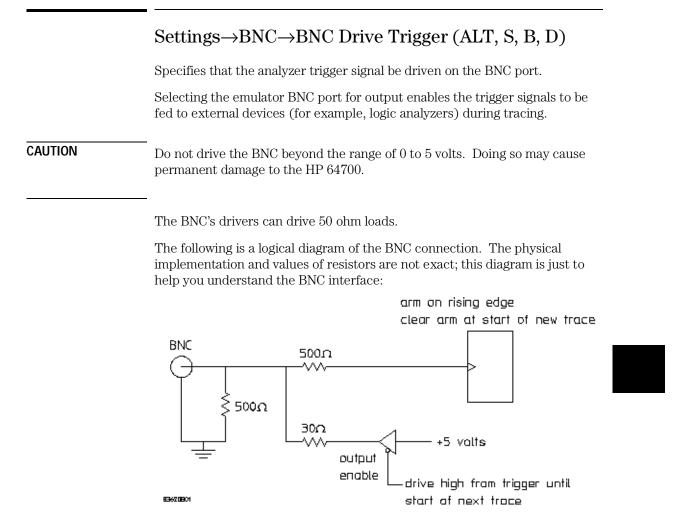
When a trace starts, it stops driving the output (so if nothing else is driving the line, it will fall low due to the 500 ohm pull-down resistor).
