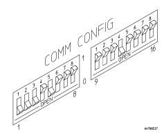
Notice that switches 1 through 3 are set to 111, respectively. This sets the baud rate to 230400.
