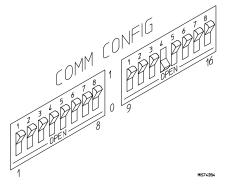
Notice that switches 12 and 13 are set to 1 and 0, respectively. This sets the RTS/CTS hardware handshake which is needed to make sure all characters are processed.
