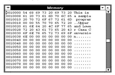
The Memory window has *control menu* commands that let you change the format of the memory display and the size of the locations displayed or modified. When the absolute (single-column) format is chosen, symbols corresponding to addresses are displayed. When data is displayed in byte format, ASCII characters for the byte values are also displayed.
