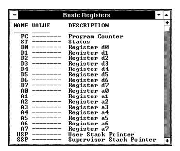
Notice that register contents are replaced with "----" in the display. This shows the debugger cannot update the register display. In order for the emulator to update its register display, the emulation monitor must interrupt target program execution while it reads the registers.
