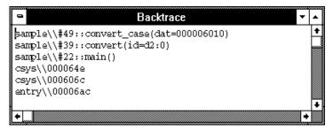
The BackTrace window is updated when program execution stops at an occurrence of breakpoint, break, or Step command.
