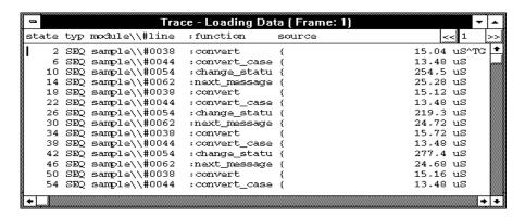
For each line in the Trace window, the trace buffer state number, the type of state, the module name and source file line number, the function name, the source line, and the time count information are displayed.
