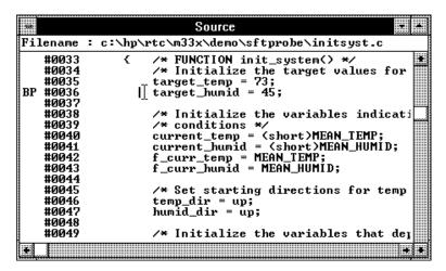
Notice that line 36 is marked with "BP," which indicates a breakpoint has been set on the line.
