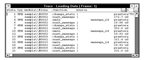
You can see how prefetching affects tracing by choosing the Display—Mixed Mode (ALT, -, D, M) command from the Trace window's control menu.
