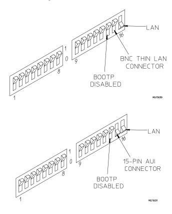
Switch 16 must be set to one (1) indicating that a LAN connection is being made.
