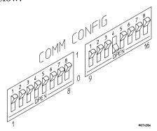
Notice that switches 12 and 13 are set to 1 and 0, respectively. This sets the RTS/CTS hardware handshake, which is needed to make sure all characters are processed. Switches 1, 2, and 3 are set to 0. This sets the baud rate to 9600. Switch settings are read during the HP 64700 power up routine.
