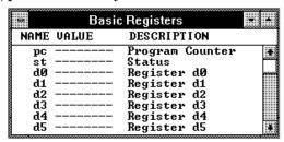
Notice that register contents are replaced with "----" in the display. This shows the debugger cannot update the register display.
