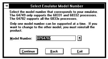
Once you have selected the correct model number, choose the Continue button. To back up to the preceding "Welcome" screen, choose the Back button. To exit the installation procedure, choose the Exit button.
