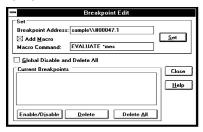
Breakpoint Displays the specified line number or address followed by a decimal point and the break macro line number.
