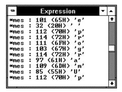
When a variable name is specified with the EVALUATE command, the Expression window displays the evaluation of the variable. When a quoted string of ASCII characters is specified with the EVALUATE command, the Expression window displays the string.
