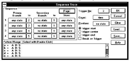
Choosing the primary branch, secondary branch, store, count, or prestore buttons opens a Condition dialog box that lets you select "any state," "no state," trace patterns "a" through "h," "range," or "arm" as the condition. Patterns "a" through "h," "range," and "arm" are grouped into two sets, and resources within a set may be combined using the "or" or "nor" logical operators. Resources in the two sets may be combined using the OR or AND logical operators.
