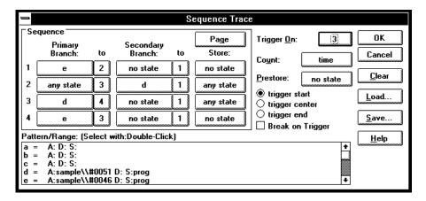
Notice that the analyzer triggers on the entry to sequence level 3. The primary branch condition in level 2 actually specifies the trigger condition.
