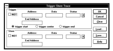
A group of Address, Data, and Status text boxes combine to form a *state qualifier*. You can specify an address range by entering a value in the End Address box. By selecting the NOT check box, you can specify all states other than those identified by the address, data, and *status values*.
