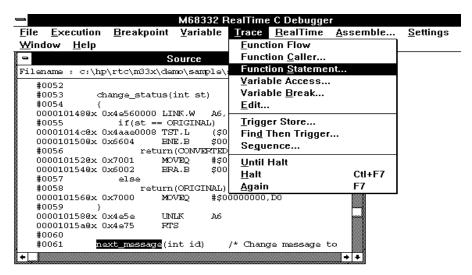
The Trace window becomes active and displays the results. You can see how prefetching affects tracing by choosing the Display—Mixed Mode (ALT, -, D, M) command from the Trace window's control menu.
