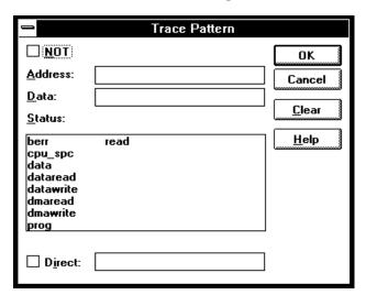
If you double-click on the range resource at the bottom of the Pattern/Range list box, the Trace Range dialog box is opened to let you select either the Address range option or the Data range option and enter the minimum and maximum values in the range.
