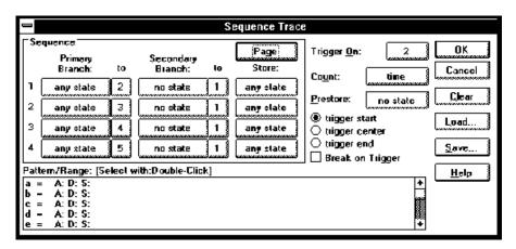
The Sequence group box specifies primary and secondary branch conditions for transferring from one sequence level to another. It also specifies store conditions for each of the eight sequence levels.
