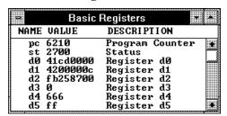
The Register window opens and displays the register contents. The display is updated periodically.
