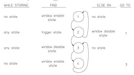
Notice that the order of the second sequence level pair is swapped. In sequence level 2, if the analyzer finds the trigger condition while searching for the window disable state, it will branch to sequence level 3 where it continues its search for the window disable state. After this, the analyzer will remain in sequence levels 3 and 4 until the trace memory is filled, completing the trace.
