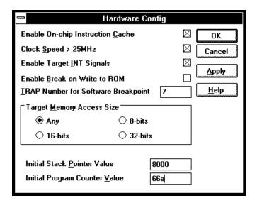
Enable On-chip Instruction Cache Lets you disable the on-chip instruction cache when you trace program execution. This causes all instruction fetches to be visible on the external bus (at the expense of processor performance).
