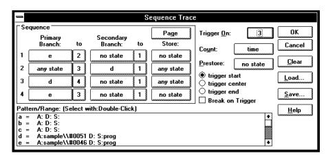
Notice that the analyzer triggers on the entry to sequence level 3. The primary branch condition in level 2 actually specifies the trigger condition.
