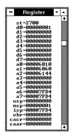
The Register window opens and displays the register contents. The display is updated periodically.
