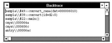
The BackTrace window is updated when program execution stops at an occurrence of a breakpoint, break, or Step command.
