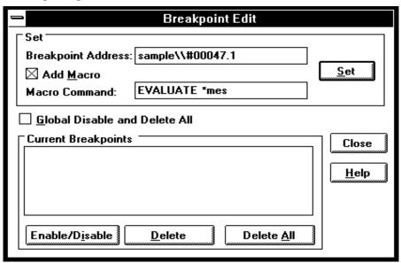
Breakpoint Address Displays the specified line number or address followed by a
