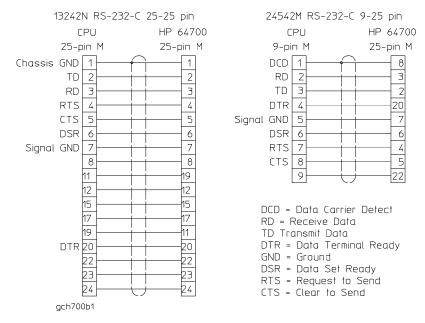
You can also use an RS-232C printer cable, but you must set HP 64700 configuration switch 4 to 1.
