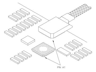
CAUTION: MAKE SURE PIN A1 OF THE PROBE CONNECTOR IS
