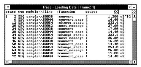
For each line in the Trace window, the trace buffer state number, the type of state, the module name and source file line number, the function name, the source line, and the time count information are displayed.
