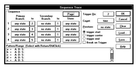
The Sequence group box specifies two types of branch conditions for transferring from one sequence level to another. It also specifies store conditions for each of sequence levels 1 through 8.
