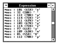
When a variable name is specified with the EVALUATE command, the Expression window displays the evaluation of the variable. When a quoted string of ASCII characters is specified with the EVALUATE command, the Expression window displays the string.
