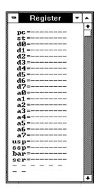
Notice that register contents are replaced with "----" in the display. This shows the debugger cannot update the register display. In order for the emulator to update its register display, the emulation monitor must interrupt target program execution while it reads the registers.
