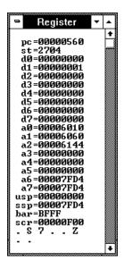
You can modify register contents by double-clicking on the register value, using the keyboard to type in the new value, and pressing the Enter key. When you double-click on the Status Register (st), System Control Register (scr), or Base Address Register (bar) values, a dialog box opens and allows you to set or clear individual bits.
