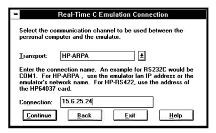
When using the HP-RS422 transport, the connection name is the I/O address you want to use for the HP 64037 card. Enter a hexadecimal number from 100H through 3F8H, ending in 0 or 8, that does not conflict with other cards in your PC.
