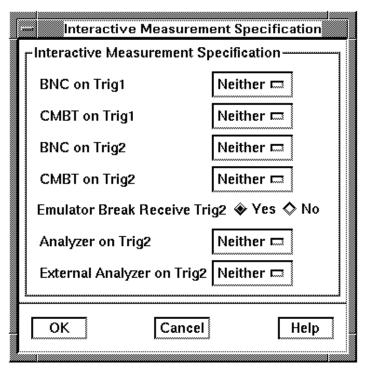
If you're using the Softkey Interface from a terminal or terminal emulation window, you don't get a dialog box from which to choose configuration sections; however, you have access to the same configuration options through a series of configuration questions. To access the questions in the "Interactive Measurement Specification" section, answer "yes" to the "Modify interactive measurement specification?" question.
