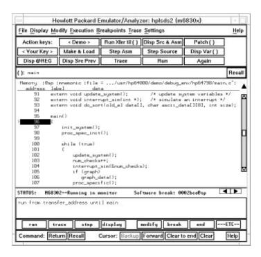
Notice the message "Software break: <address>" is displayed on the status line and that the emulator is "Running in monitor" (you may have to click the *select* mouse button to remove temporary messages from the status line). When you run until an address, a breakpoint is set at the address before the program is run.
