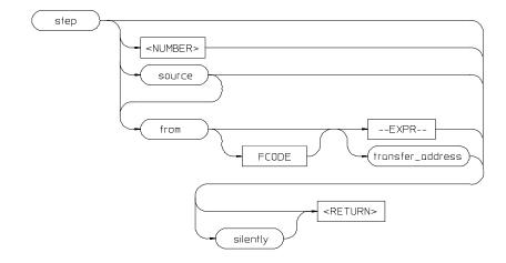
The **step** command allows sequential analysis of program instructions by causing the emulation processor to execute a specified number of assembly instructions or source lines.
