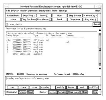
Notice the entry labeled "info". Ranges with this label do not take up mapper resources; they just show information about the processor's address space. Another "info" entry will be listed if the internal RAM is enabled with the EMRAMBAR register.
