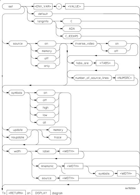
Controls the display format for the data, memory, register, software breakpoint, and trace displays. With the **set** command, you can adjust the display format results for various measurements, making them easier to read and interpret. Formatting of source lines, symbol display selection and width, and update after measurement can be defined to your needs.
