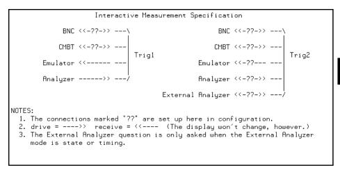
Note that the "External Analyzer" connection for "Trig2" is only available if you have selected "state" or "timing" for the external analyzer mode.
