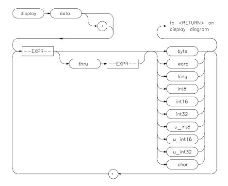
This command can display the values of simple data types in your program. Using this command can save you time; otherwise, you would need to search through memory displays for the location and value of a particular variable.
