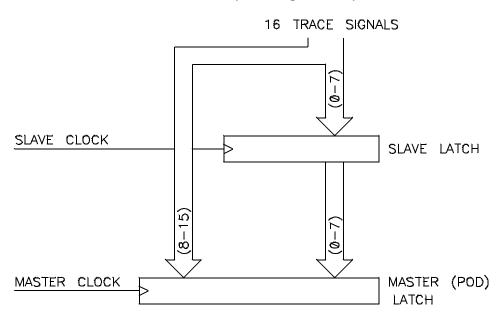
If no slave clock has appeared since the last master clock, the data on the lower 8 bits of the pod will be latched at the same time as the upper 8 bits. If
