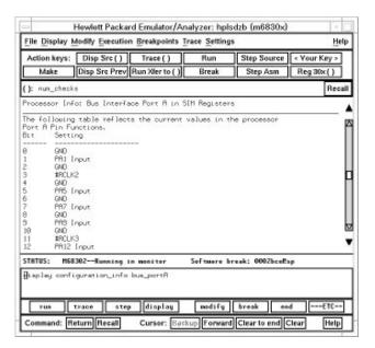
To display information about bus interface port A from the emsim (emulator) register set, choose **Display**—**Configuration Info**—**Bus Interface Port A (Emulator SIM)** from either the configuration interface the emulator/analyzer interface pull-down menu.
