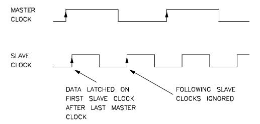
Choose "demux" to specify the true demultiplexing mode. In this mode, only the lower eight external channels (0-7) are used. The slave clock (as specified by your answers to the next four questions) latches these bits and the emulation clock samples the same channels again. The latched bits show up as bits 0-7 in the trace data, and the second sample shows up as bits 8-15 (see the figure below).
