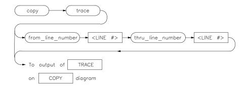
This command copies the contents of the trace buffer to a file or to the printer.
