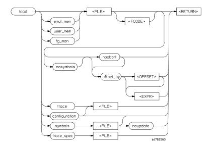
This command transfers absolute files from the host computer into emulation or target system RAM. With other parameters, the *load* command can load emulator configuration files, trace records, trace specifications, or symbol files.
