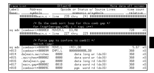
Notice in the resulting trace (you have to press the <NEXT> key) that the enable and disable states have the "sq adv" string in the line number column. This is because the windowing feature uses the analyzer's sequencer.
