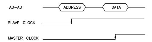
If no slave clock has appeared since the last master clock, the data on the lower 8 bits of the pod will be the same as the upper 8 bits. If more than one slave clock has appeared since the last master clock, only the first slave data will be available to the analyzer.
