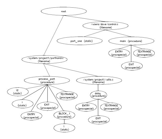
Note that SRU does not build tree nodes for variables that are dynamically allocated on the stack at run-time, such as i and j within the delay () procedure. SRU has no way of knowing where these variables will be at run
