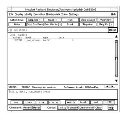
The "num\_checks" variable is added to the data values display and its value is displayed as a 32-bit integer.
