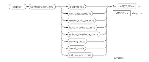
This command displays information about emulator configuration and processor SIM programming. You can also display diagnostic information about inconsistencies found in the emulator configuration.
