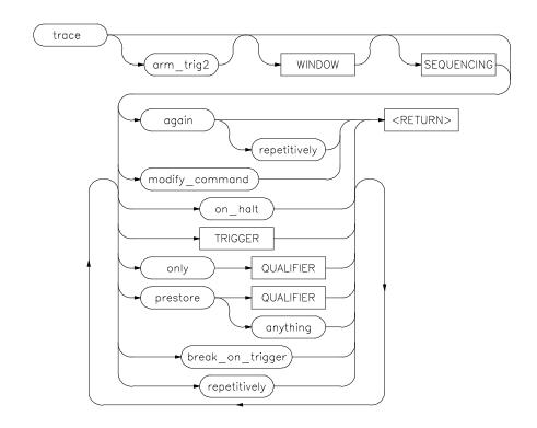
This command allows you to trace program execution using the emulation analyzer.
