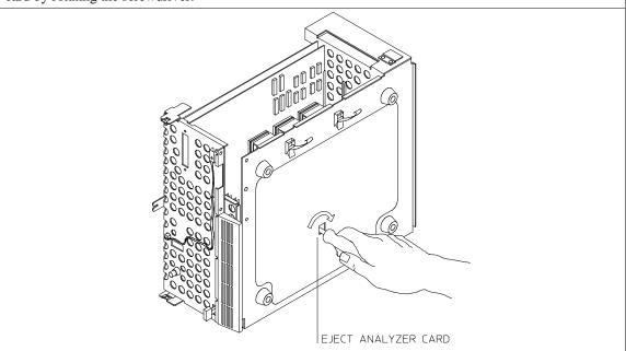
Do not remove the system control board. This board is used in all HP 64700 emulation and analysis systems.
