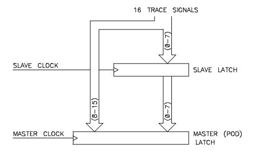
If no slave clock has appeared since the last master clock, the data on the lower 8 bits of the pod will be latched at the same time as the upper 8 bits. If more than one slave clock has appeared since the last master clock, only the first slave data will be available to the analyzer (see the figure below).
