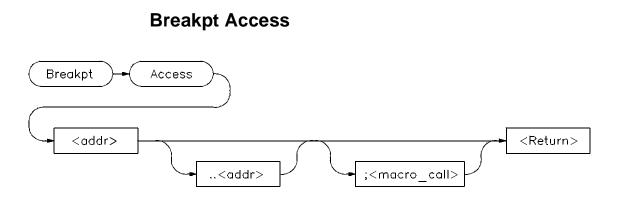
The Breakpt Access command sets an access breakpoint at the specified memory location (<addr>) or range (<addr>..<addr>). The access breakpoint halts program execution each time the target program attempts to read from or write to the specified memory location or range. Memory locations may contain code or data.
