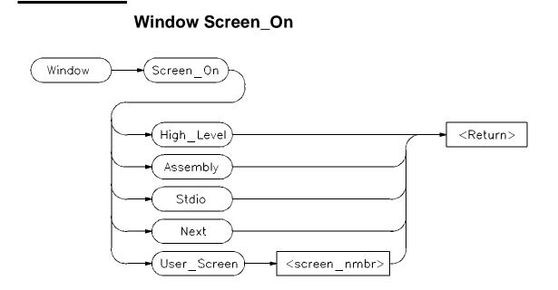
The Window Screen\_On command displays the selected screen. You can also use function key *F6* to display a screen.
