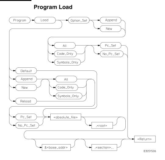
The Program Load command loads and reloads the specified executable module into the debugger and also allows you to set default options for loading executable modules.
