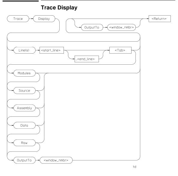
The Trace Display command displays trace information in the specified window. If no window is specified, the trace output will go to the Trace Mode window, and the debugger willl enter "trace mode."
