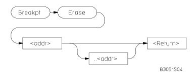
The Breakpt Erase command erases (deletes) a previously set breakpoint at a specific address or all breakpoints set within a range of addresses. The Breakpt Erase command differs from the Breakpt Delete command in that you identify the breakpoint(s) you wish to remove by an address or by a range of addresses instead of by a breakpoint number.
