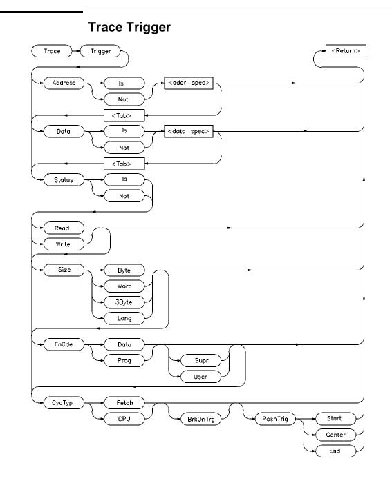
The Trace Trigger command specifies the bus conditions to be used as the trigger condition. Bus conditions may be address values, data values, or status values. When you define a trigger, you are essentially defining an event. You can also use the *Trace Event Specify* command to define an event, and then use the *Trace Trigger Event* command to use the specified event as the trigger event.
