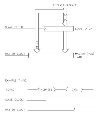
If no slave clock has appeared since the last master clock, the data on the lower 8 bits of the pod will be the same as the upper 8 bits. If more than one slave clock has appeared since the last master clock, only the first slave data will be available to the analyzer.
