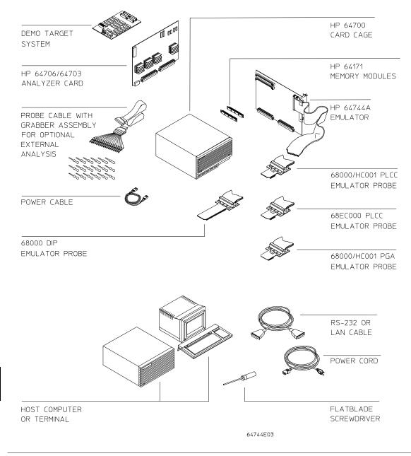
The HP 64744 68000/HC001/EC000 Emulator card and the HP 64706/3 Emulation Bus Analyzer card, when installed into the HP 64700 Card Cage, are used for emulation and analysis of 68000/HC000/HC001/EC000 microprocessor systems.
