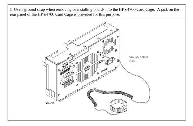
When removing or installing cards, you should use a ground strap to reduce the chances of damaging circuit cards from static discharge.
