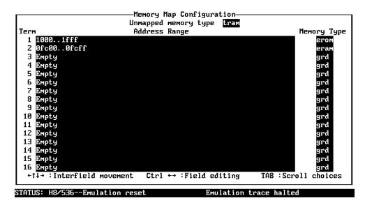
Use the TAB and Shift-TAB keys to pick memory type for mapped range.
