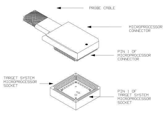
Figure 3-8. Installing into a PLCC type socket
