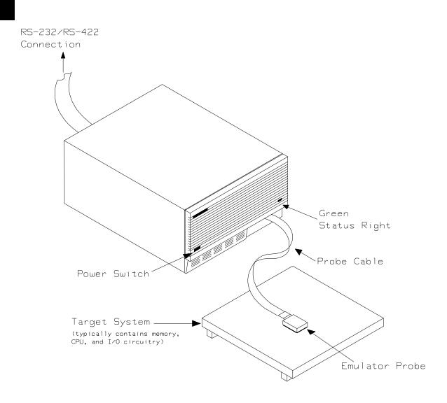
Figure 1-1. HP 64739 Emulator for the H8/536 Processor
