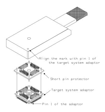
Figure 3-1. Installing the Target System Probe
