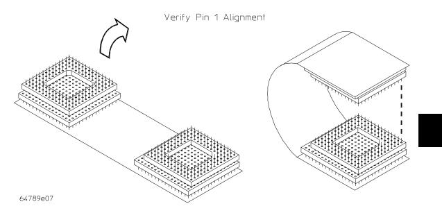
The Flexible Cable has a 15 X 15 pin arrangement, and the 80386 emulator uses a 14 X 14 pin arrangement. Verify proper alignment of the socket, male header, and Flexible Cable. You might paste a paper dot on the Flexible Cable to mark pin 1 on both connectors before connecting the Flexible Cable between the emulator probe and the target microprocessor.
