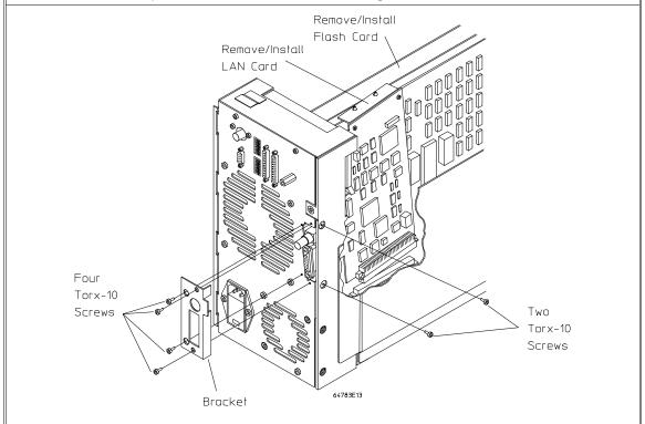
14 This step applies only to the HP 64700A. If you wish to install the flash card (used for updating firmware, see chapter 5), refer to the diagram above. Install the flash card in any available slot between the 80-channel analyzer card and the HP 64748C control card in the cardcage. Insert the flash card in the plastic guides. Make sure the connectors are properly aligned. Then press the card all the way into the mother board sockets.
