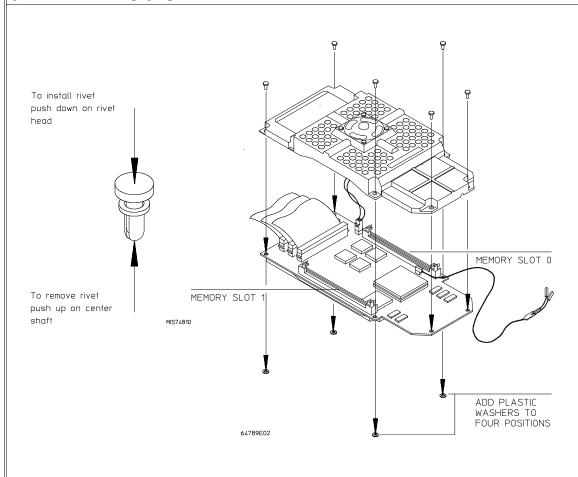
2 Determine the placement of the emulation memory modules. Three types of modules may be installed: 256 Kbyte (HP 64172A), 1 Mbyte (HP 64172B), and 4 Mbyte (HP 64173A). Any of the emulation memory modules can be installed in either memory slot on the probe.
