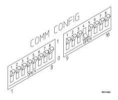
Switches 12 and 13 are set to 1 and 0, respectively. This sets the RTS/CTS hardware handshake, which is needed to make sure all characters are processed.
