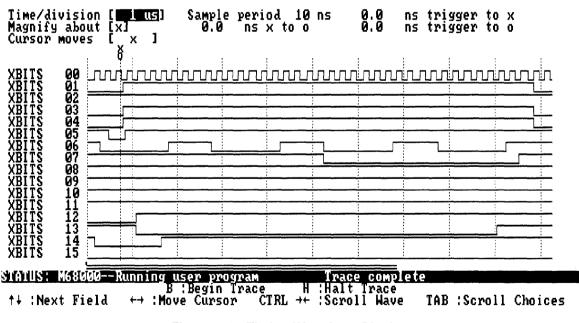
Figure 5-9. Timing Waveform Display
