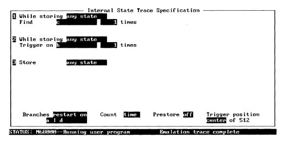
Use the TAB and Shift-TAB keys to select a trigger position or enter a number.
