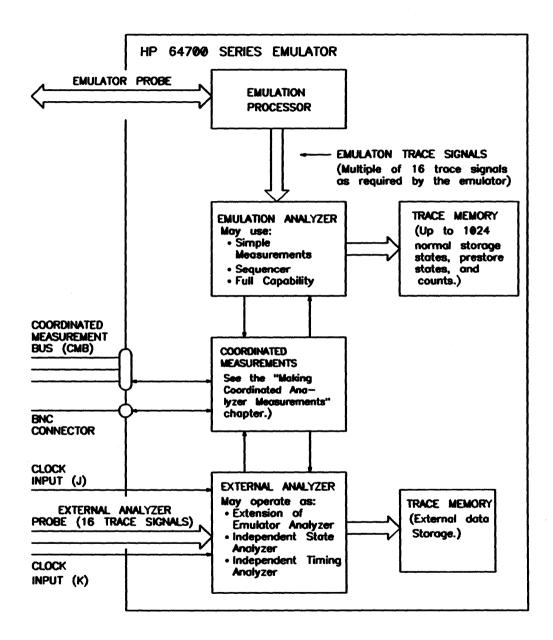
Figure 1-1. Block Diagram of HP 64700 Series Analyzer
