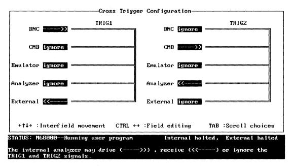
Figure 6-2. Receiving External Signals
