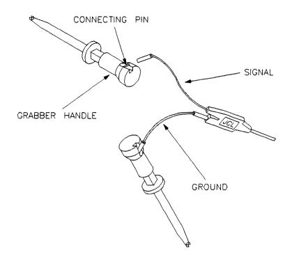
Figure 4-2. Attaching Grabbers to Probe Wires
