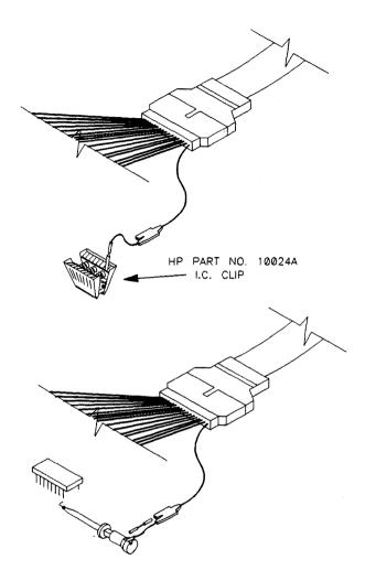
Figure 4-5. Connecting the Probe to the Target System
