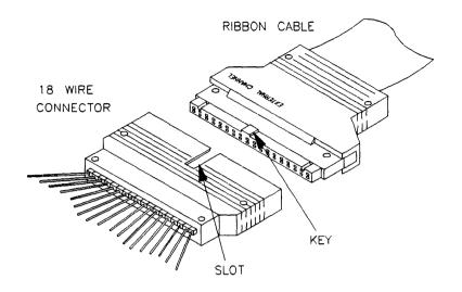
Figure 4-1. Assembling the Analyzer Probe
