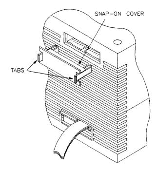
Figure 4-3. Removing Cover to Emulator Connector
