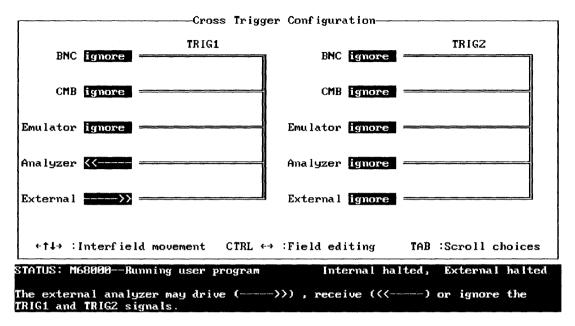
Figure 6-3. Using One Analyzer to Arm the Other
