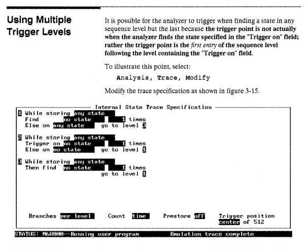
Use the TAB and Shift-TAB keys to select a trigger position or enter a number.
