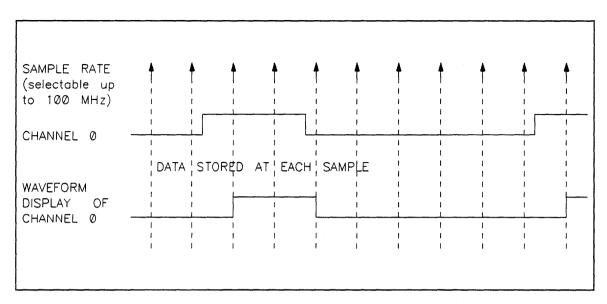
Figure 5-4. Standard Acquisition Mode
