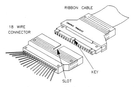
Figure 4-1. Assembling the Analyzer Probe
