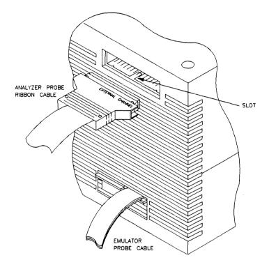
Figure 4-4. Connecting the Probe to the Emulator
