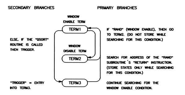
Figure 3-6. Tracing a "Window" of Activity
