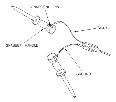
Figure 4-2. Attaching Grabbers to Probe Wires
