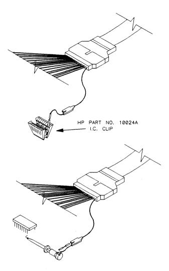
Figure 4-5. Connecting Probe to the Target System
