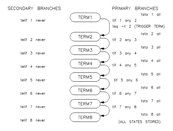
Figure 3-2. "Complex" Configuration Default Sequencer
