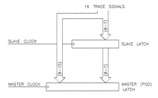
Figure 6-2. Mixed Clock Demultiplexing
