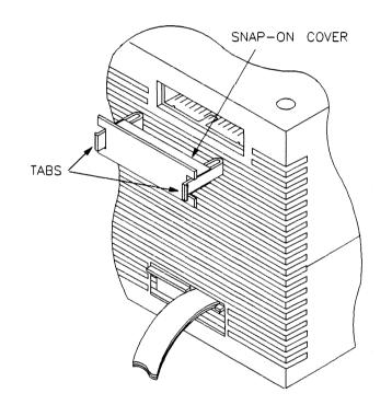
Figure 4-3. Removing Cover to Emulator Connector
