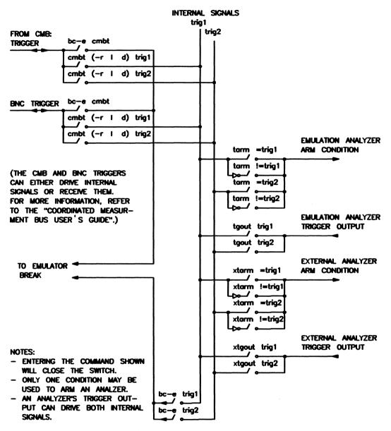
Figure 5-1. Coordinated Measurements
