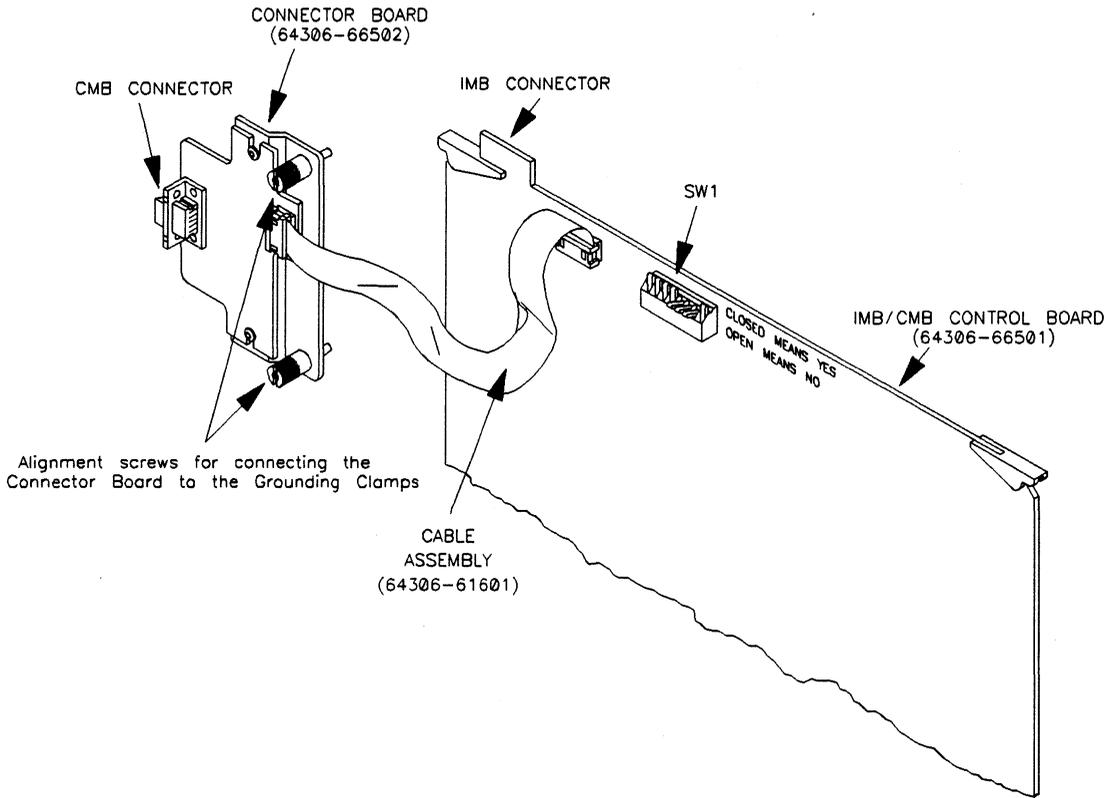
Figure 5-2. HP 64306A IMB/CMB Interface Boards
