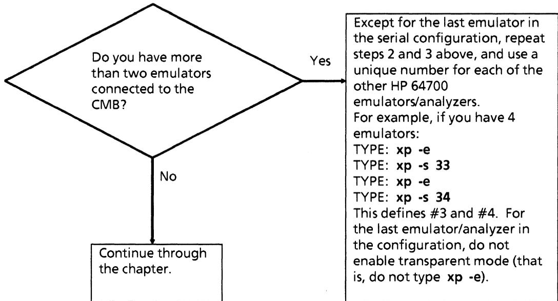
Figure 4-2. How Many Emulators Are Connected To CMB?
