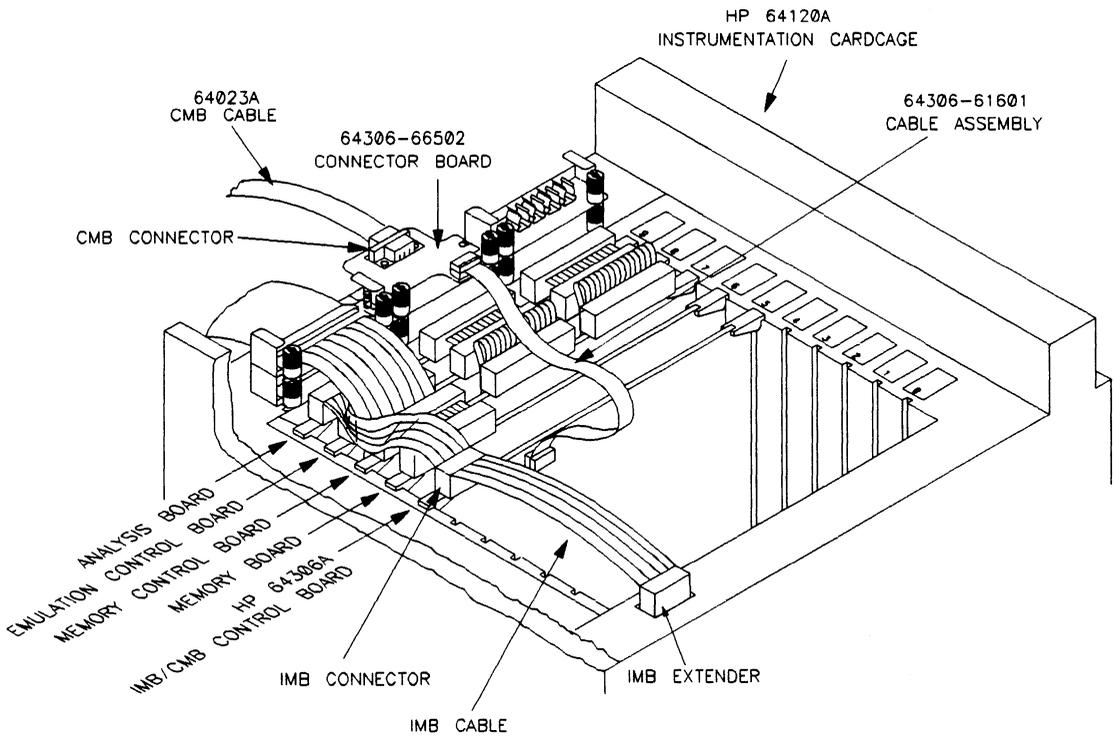
Figure 5-4. HP 64306A In A Complete System
