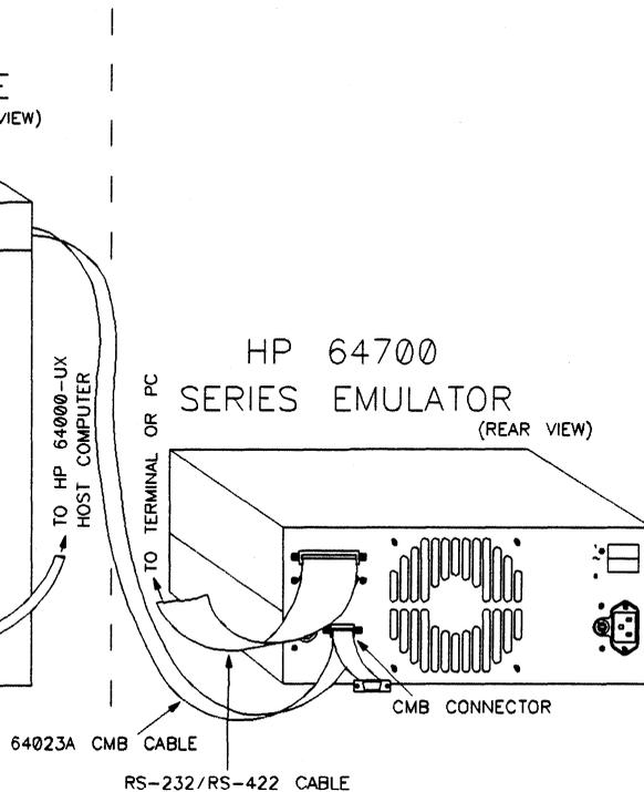
Figure 5-1. IMB/CMB Connections
