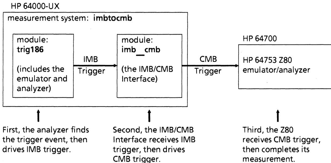
Figure 5-5. HP 64000-UX Drives Trigger To HP 64700
