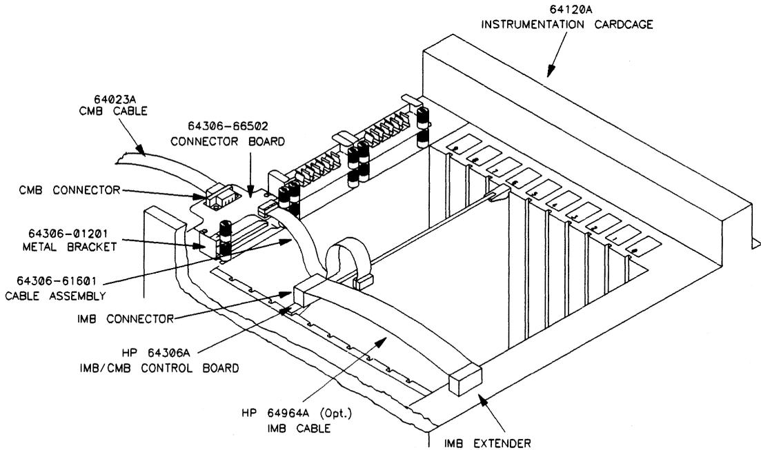
**Figure 5-3. HP 64306A Installed In HP 64120A**
