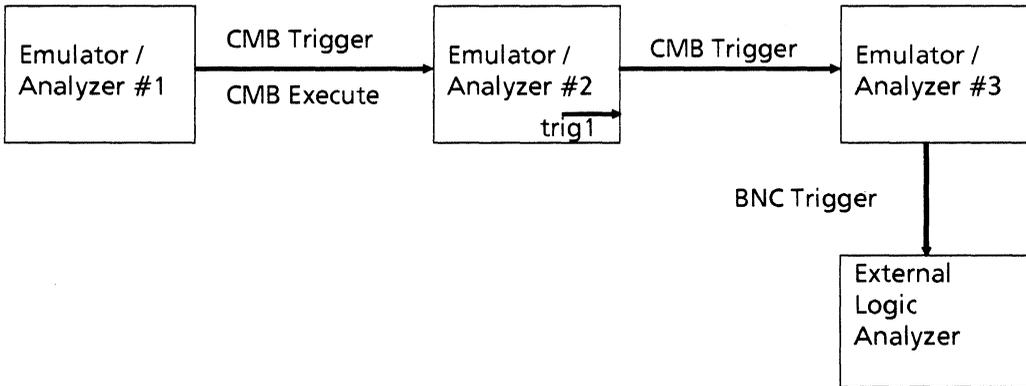
Figure 4-4. Measurements Between Several Emulators
