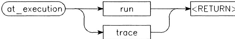
**Function** **at\_execution** is used to prepare a run or trace command for execution. This command is used in conjunction with the execute command. If the processor is not reset, **at\_execution run** causes a break from your program, and initializes the monitor to the default address or to the specified address. An execute command then causes the run to occur. Once an execution has occurred, the run specification is removed and cannot be repeated without respecifying the run.
