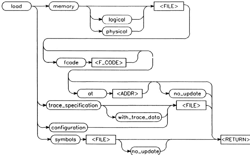
**Function** The load memory command transfers absolute code from the host system disc into target system RAM or emulation memory. The destination of the absolute code is determined by the memory configuration map which was set up during emulation configuration and the address specified during linking.
