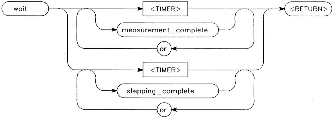
**Function** The wait command is a delay command. Delay commands are enhancements that allow flexible use of command files (although delays are also available outside of command files). Command delays give the emulation system and target processor time to reach some condition or state before bringing in the next command. The delay commands may be included in command files.
