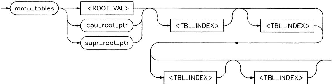
**Function** The **display mmu\_tables** command displays the translation table entries at a given level. The tables will be indexed from the given root pointer using the index values. These values will not be checked for validity (that is, if an index goes past the end of that level, this will not be an error if the resulting value is a table entry).
