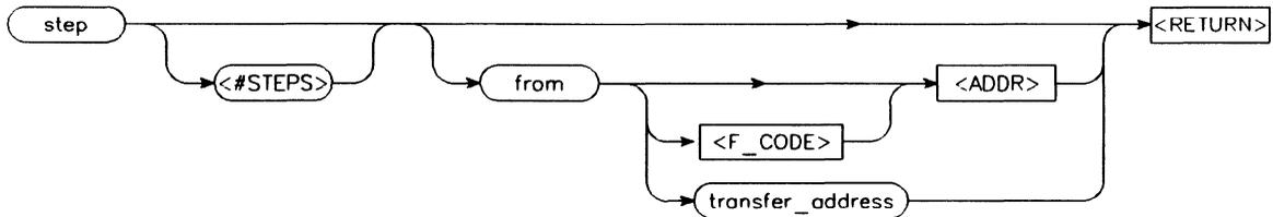
**Function** The step command allows program instructions to be sequentially analyzed by causing the emulation processor to execute a specified number of instructions. The contents of the processor registers, the contents of trace memory, and the contents of emulation or target memory can be displayed after each step command has been completed.
