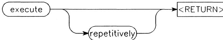
**Function** The execute command starts a trace measurement. The execute softkey label is replaced with the halt softkey label when a measurement is in progress. If emulation is participating in a system measurement through cross-triggered analysis or the emulation start function (at\_execution run or at\_execution trace), then the system measurement is initiated. Otherwise, the execute command is not available.
