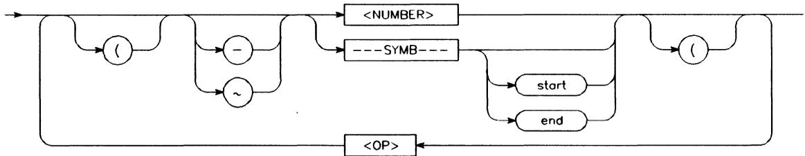
**Function** An expression is a combination of numeric values, symbols, operators, and parentheses specifying an address, data, status, or any of several other value types used in the emulation commands.
