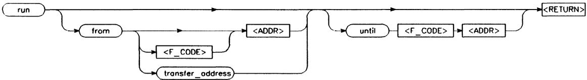
**Function** If the processor is in a reset state, run will cause the reset to be released, and if a "from" address is specified the processor will be directed to that address. If the processor is running in the monitor, the run command causes the processor to exit into your program. The program can either be run from a specified address (--EXPR--), from the address currently stored in the processor's program counter, or from a label specified in the program.
