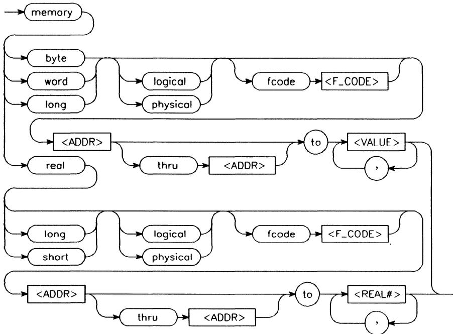
**Function** The modify memory command enables you to modify the contents of selected memory locations. The command can modify the contents of each memory location in a series to an individual value or the contents of all of the locations in a memory block to a single or repeated sequence of values.
