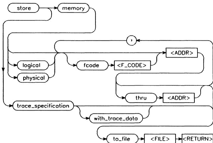
**Function** The store command is used to store the contents of specific memory locations into an absolute file (.X file), or to store the trace specification, with or without trace data, into a trace file (.TR file).
