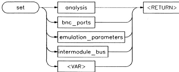
**Function** The set command is used to change the configuration for analysis, the bnc ports, or the intermodule bus; to modify emulation timeout; or to set up environmental variables.
