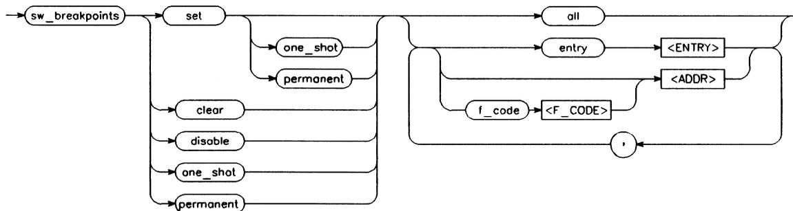
**Function** Software breakpoints enables the emulator to "break on execution" of a specified address. Any valid address (number, label or expression) may be specified as a breakpoint. Valid addresses identify the first word of valid instructions.
