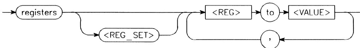
**Function** The modify register command is used to modify the contents of one or more registers in the processor/coprocessor's register set. The entry for <REG> determines which register is modified.
