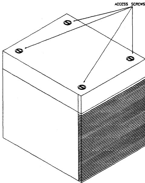
**Figure 2-2. Removing the Cardcage Access Cover**
