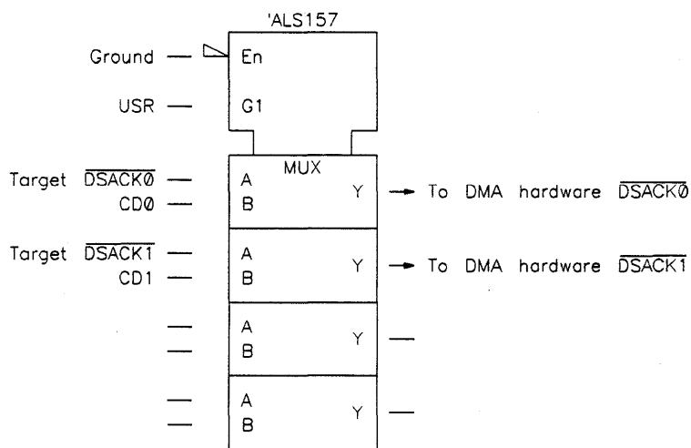
**Figure 5-3. Circuit For DMA Transfers**
