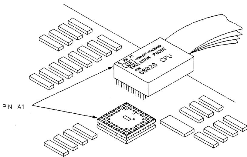
Figure 2-5. Installing Emulator Probe Into PGA Socket
