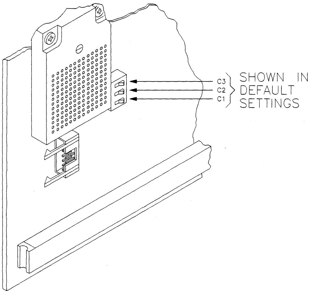
Figure 4-5. Setting Configuration Switches
