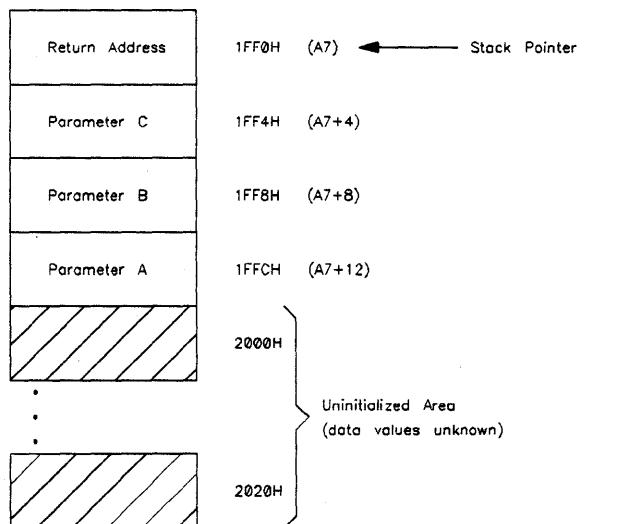
Figure 5-5. Example Stack Frame
