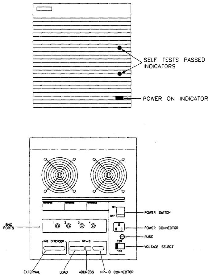
Figure 2-1. HP 64120A Instrumentation Cardcage Features
