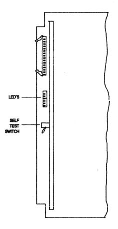
Figure 5-1. DCU Selftest Control & Indicators
