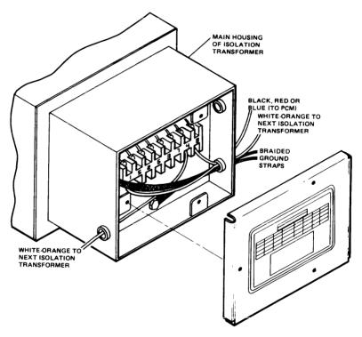
Figure 6-1. Transformer Strapping
