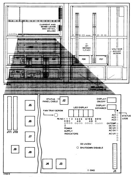
Figure 3-9. Power Supply Control Layout (HP 32460A)
