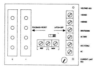
Figure 6-4. Rear View Of Power Supply (HP 32460A)
