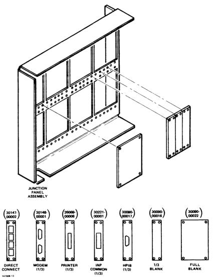
Figure 3-5. Junction Panel Assembly and Mounting Panels
