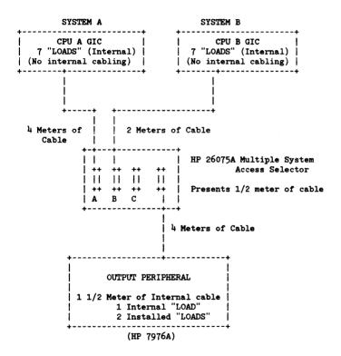
SYSTEM A CABLE LENGTH 4 Meters from GIC to HP 26075A 1/2 Meters HP 26075A Internal 4 Meters from HP 26075A to peripheral 1 1/2 Meters peripheral internal
