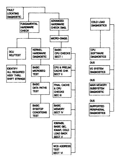
Figure 5-3. Fault Locating Diagnostic Block Diagram
