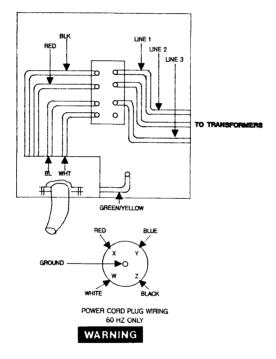
Hazardous voltages are present when the cover plate is removed. Set branch breaker to OFF. Failure to comply can result in injury or death!
