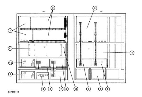
Figure 8-3. CPU and I/O Card Cages Series 64/68 (HP 32460A) Rear View
