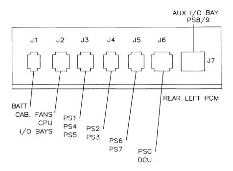
Figure 1-5. PCM Cable Connections (HP 32460A)
