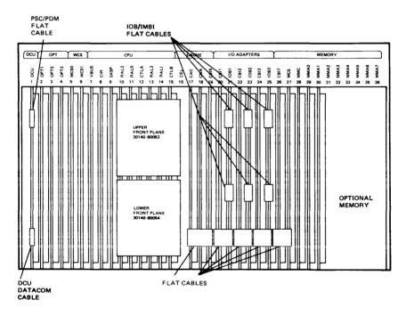
Figure 3-1. CPU Cage and Cabling Assignment
