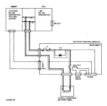
Solid line = charge path Broken line = discharge path Figure 6-8. Battery Backup System (HP 32460A)
