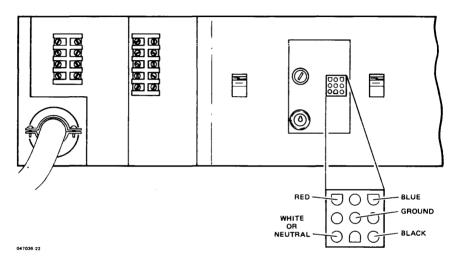
Figure 6-3. Transformer Voltage Test Points (HP 32460A)
