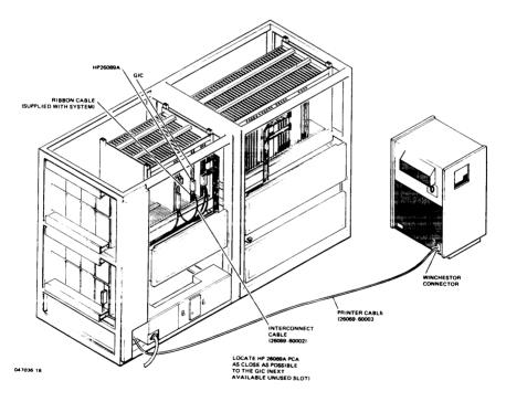
Figure 7-8. HP 2611A/13A/2617A/2619A Printer Installation
