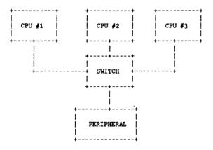
The HP 26075A is equivalent to less than 0.5 meter of standard HP-IB cable and represents no loads for HP-IB I/F.
