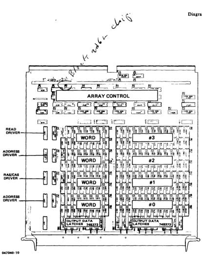
Figure 9-4. Memory Array Layout
