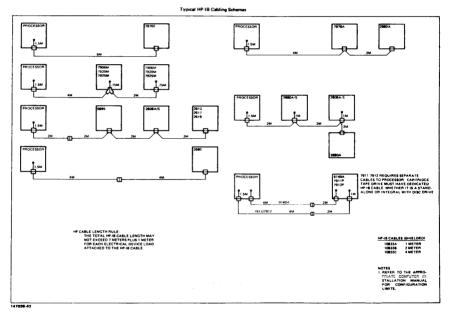
Figure 7-1. Internal HP-IB Cable Configurations
