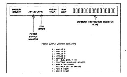
Figure 6-11. System Status Panel Display (SSPD-B)
