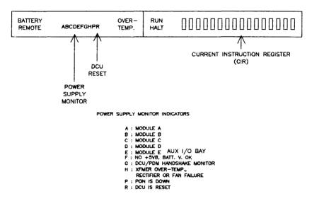
Figure 1-3. System Status and Display Panel (HP 32460B/32468B)
