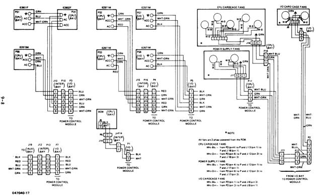
Figure 9-8 . AC Wiring (32460A)
