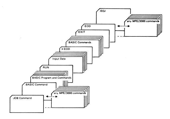
If no input data is required, the input data cards are omitted, but > EOD is left. The > EOD card must follow the input data of each run.
