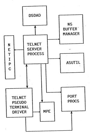
Figure 4 - Remote TELNET Module Interfaces
