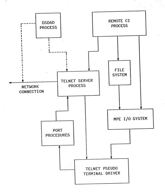
Figure 2 - TELNET Remote Structure
