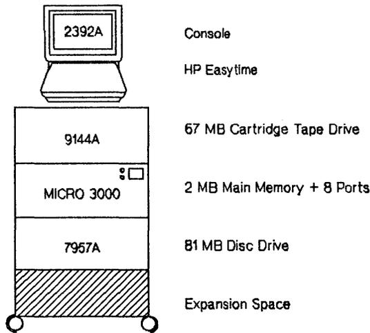
**Entry Level System (32535E).** The MICRO 3000 Entry Level System (32535E) includes the following hardware:
