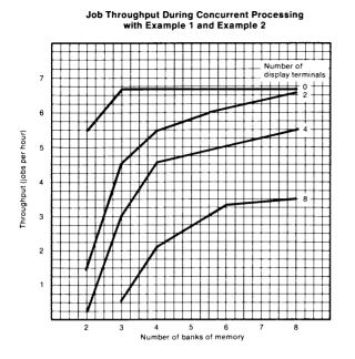
As the number of terminals (half of the terminals performing Example 1 and half performing Example 2) increases, the total throughput of the standard job, running at a lower priority, decreases as shown in the graph above. (Running two standard jobs concurrently with no terminals on an HP 300 with four banks of memory, increased throughput from 6.7 to 9.2 jobs per hour.)
