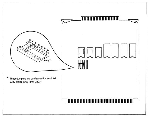
Fig. 2-2. RCM Configuration Jumper Positions
