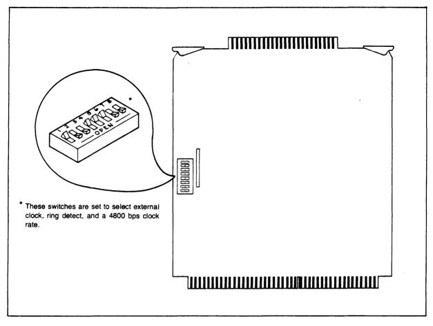
Figure 2-3. DIP Switch Position and Configuration
