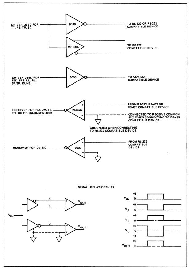
Figure 4-2. Driver/Receiver Combinations
