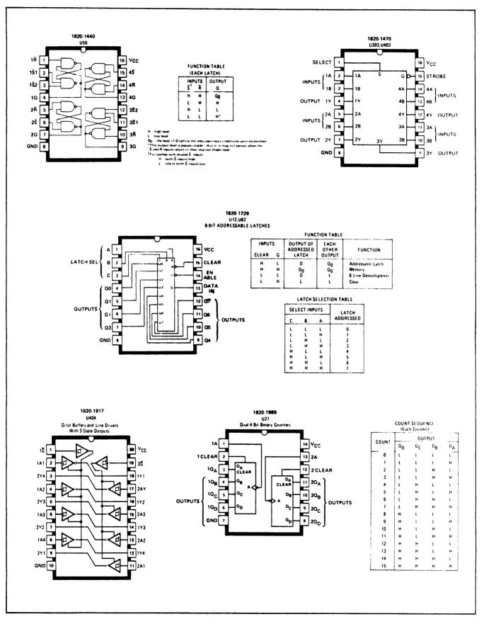
Figure 7-1. Integrated Circuit Base Diagrams (Continued)
