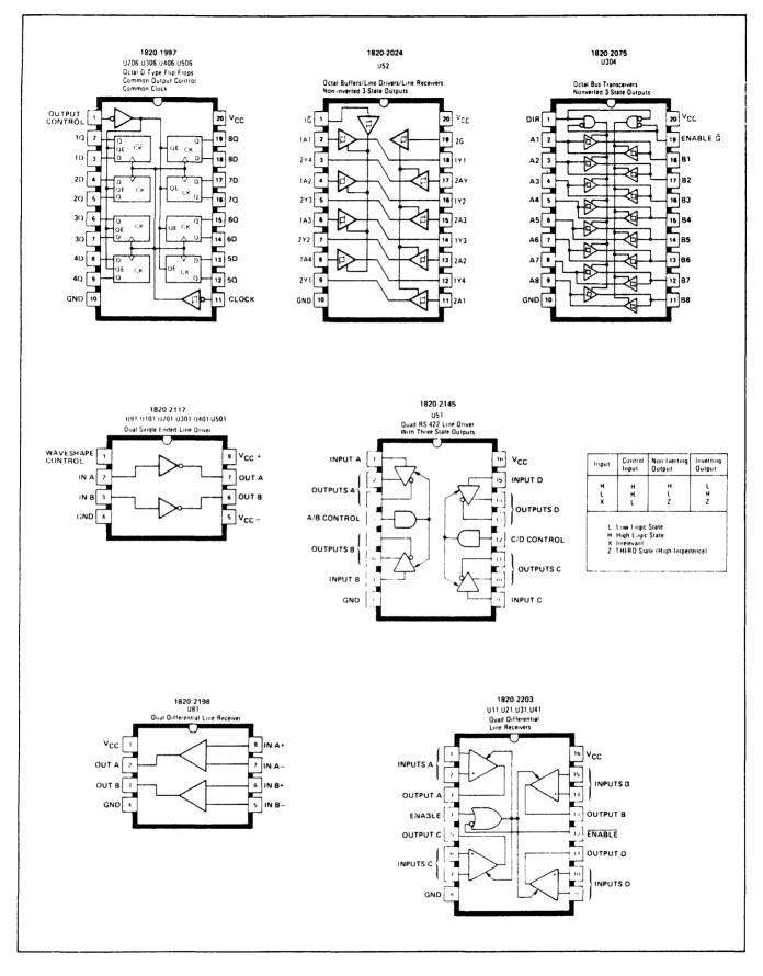
Figure 7-1. Integrated Circuit Base Diagrams (Continued)
