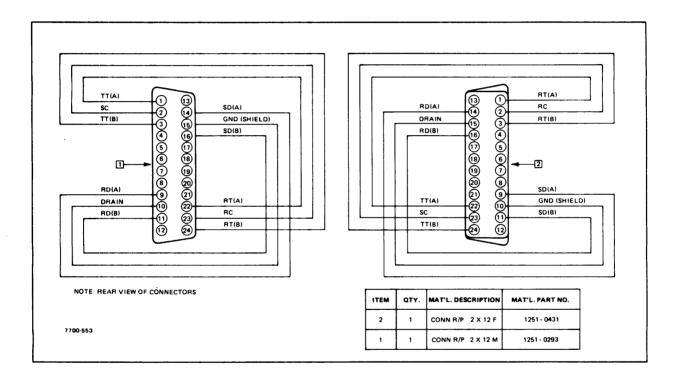
Figure 7-3. Loop-Back Test Connector Wiring Diagram.
