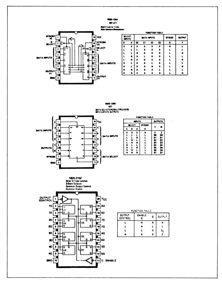
Figure 7-4. Integrated Circuit Base Diagrams (Continued)
