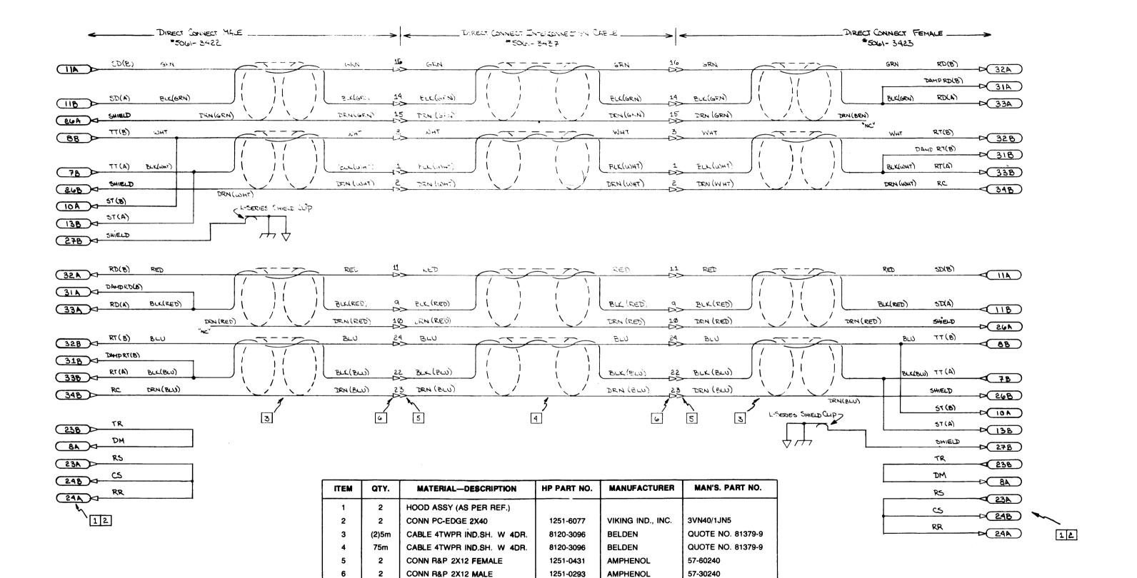
Figure 7-2. Direct-Connect Cable Wiring Diagram. 7-9/7-10
