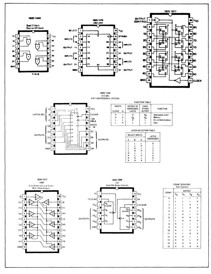
Figure 7-4. Integrated Circuit Base Diagrams (Continued)
