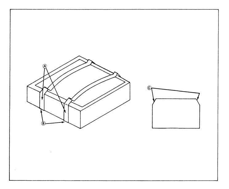
Figure 5-1. IOP Chip Socket With Retaining Clips
