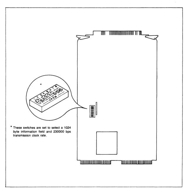
Figure 2-3. DIP Switch Position and Configuration
