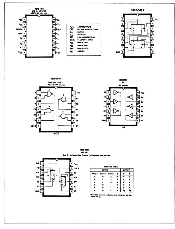
Figure 7-4. Integrated Circuit Base Diagrams.
