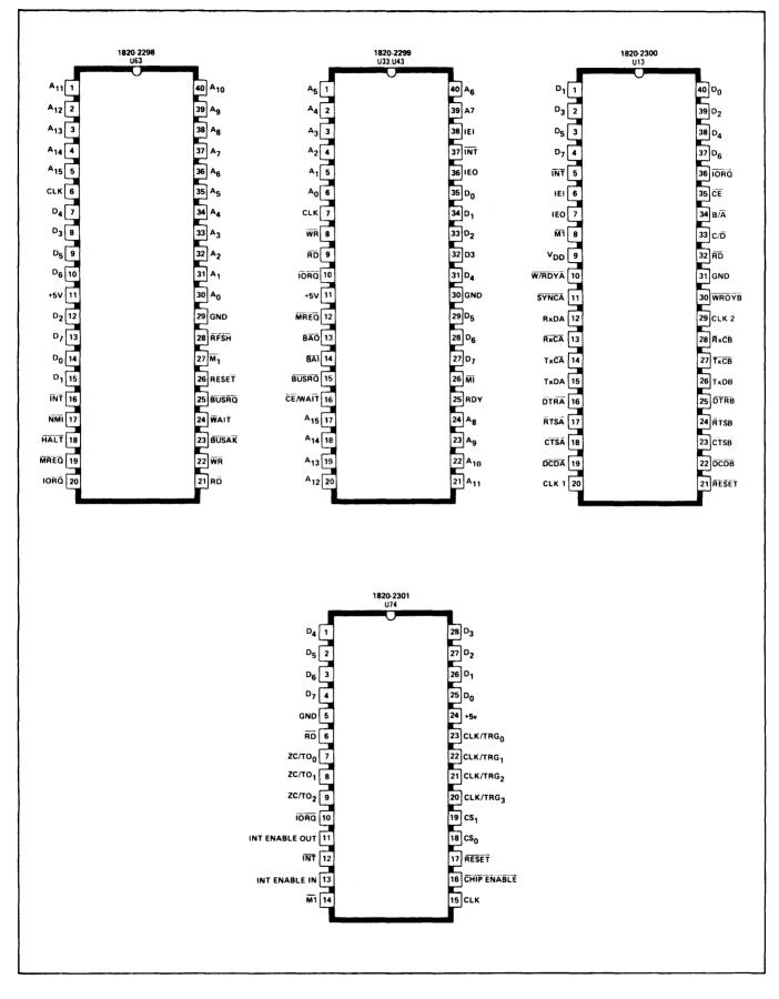
Figure 7-4. Integrated Circuit Base Diagrams (Continued)
