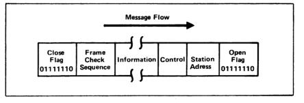
Figure 3-1. HDLC Frame Format
