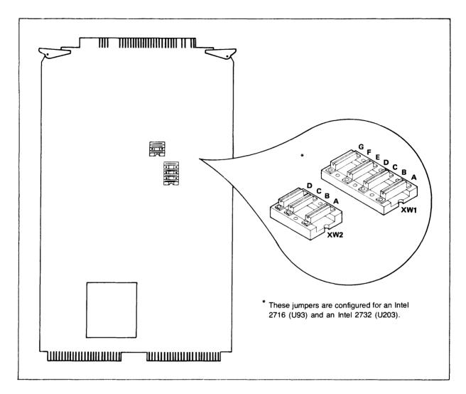
Fig. 2-2. ROM Configuration Jumper Positions
