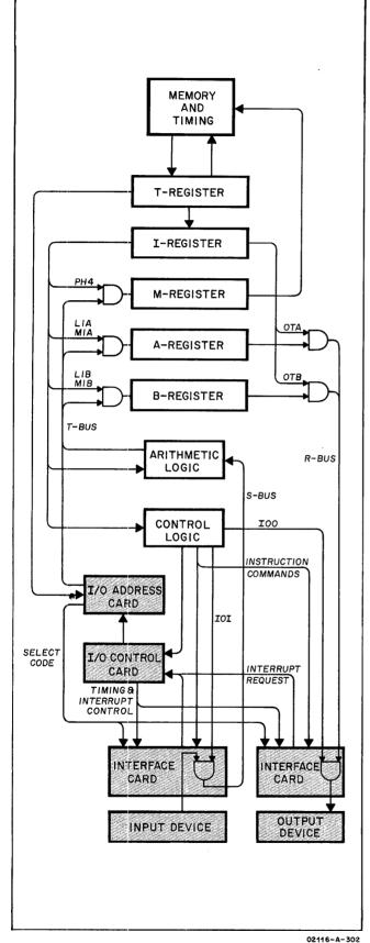
Figure 2-2. Block Diagram of System Input/Output Operations
