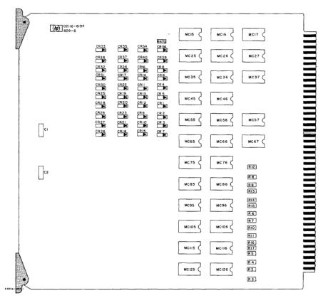
Figure 4-3. I/O Address Card, Component Location
