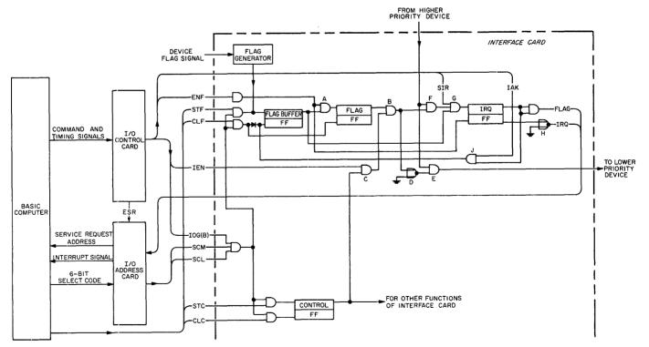
Figure 2-5. Typical Interrupt Logic
