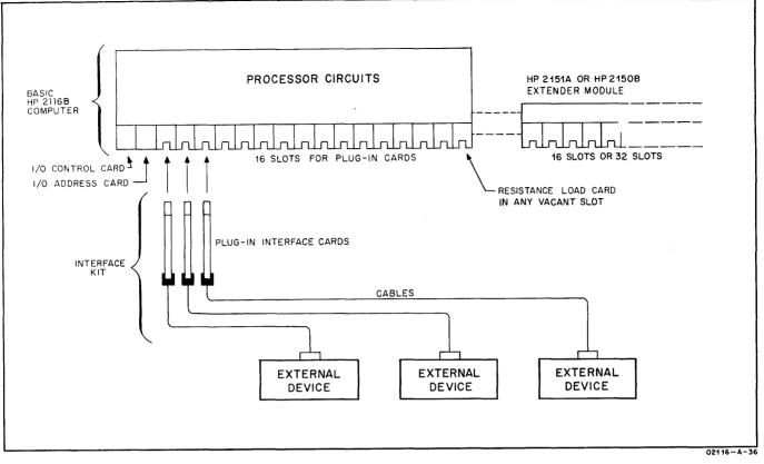
Figure 2-1. Input/Output Structure
