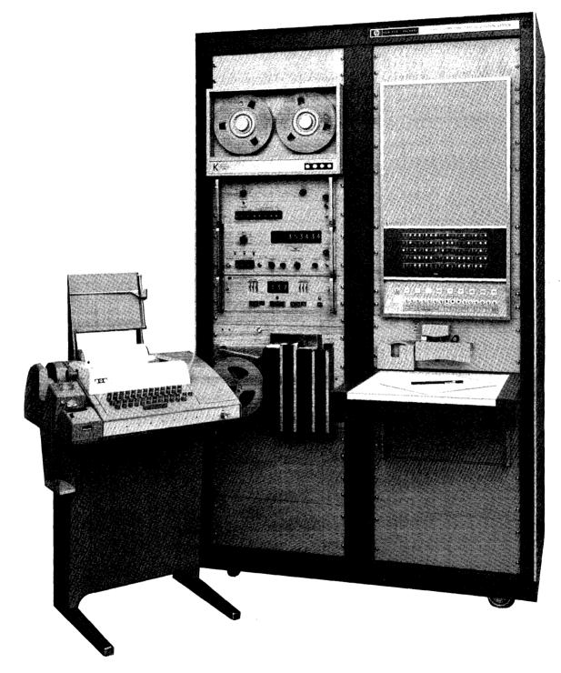
Figure 1-1. Typical HP 2116B Computer System
