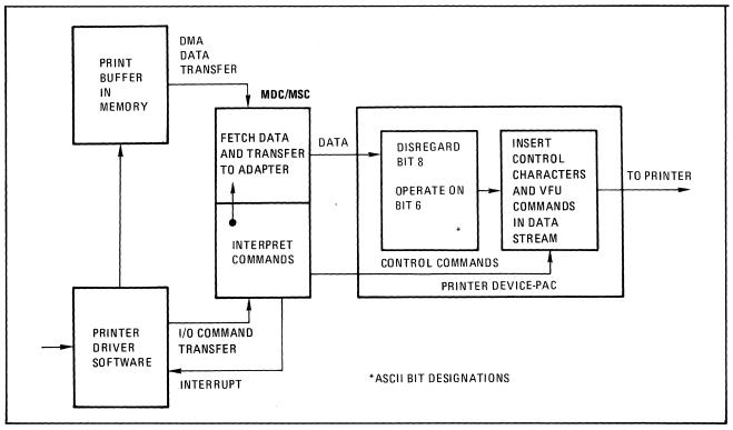
Figure 6-22. Data Manipulation of Printer Device-Pac
