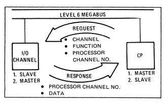
Figure 2-10. I/O Input Command
