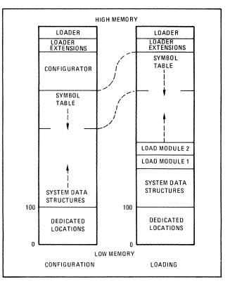
Figure 7-6. Memory Layouts During Operation of CLM
