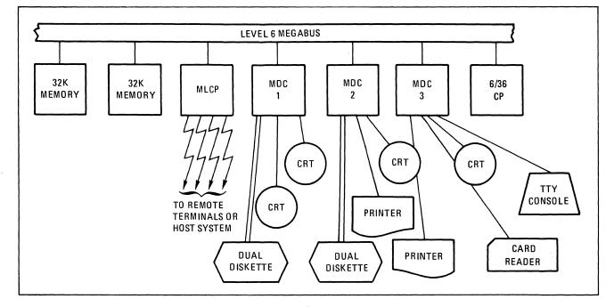
Figure 2-1. Typical 6/36 Configuration Diagram
