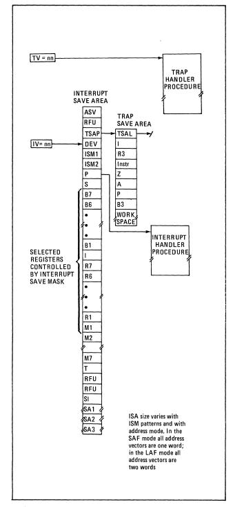
Figure 3-6. Trap Vector and Interrupt Vector Linkage
