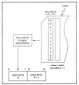
Figure 6-4. ASCII Mode Format
