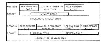
Figure 2-6. Timing of Memory Read Operation
