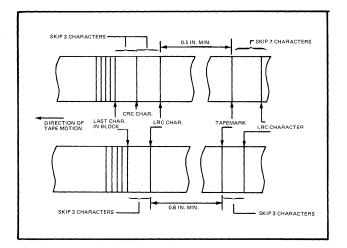
Figure 6-28. Tape Mark Block Formats
