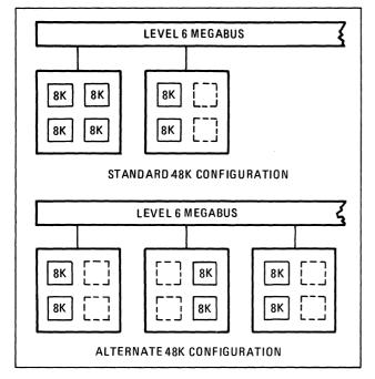
Figure 2-2. Memory Configurations
