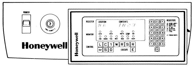
Figure 5-5. Portable Plug-in Panel Option (Shown with 6/30 Panel Plugged into Basic Panel)
