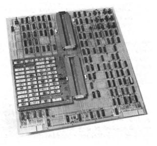
Figure 1-3. Level 6 Circuit Board (Memory Controller with 8K-Word Memory-Pac)
