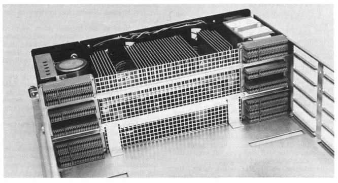
Figure 1-4. Level 6 Megabus and Power Supply
