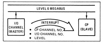
Figure 2-11. Interrupt Cycle
