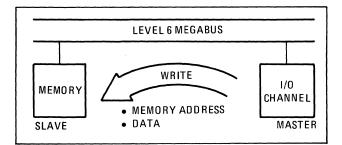
Figure 2-7. I/O DMA Input Operation
