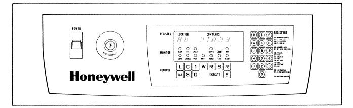
Figure 5-1. Full Control Panel (Shown with 6/40 Panel)
