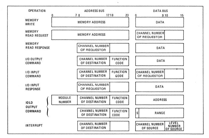
Figure 2-13. Data and Address Bus Formats
