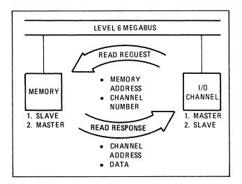
Figure 2-8. I/O DMA Output Operation
