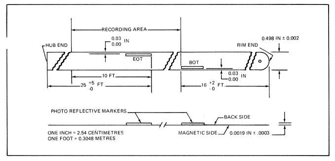
Figure 6-26. Magnetic Tape Layout
