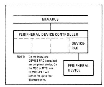
Figure 6-1. Peripheral Device Connection
