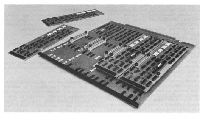
Figure 1-8. MLCP with Communications-Pacs Attached
