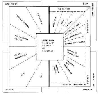
The supervision function performs job control, program loading, and multiprogram control. Job control effects automatic transition from one job to the next. Program loading encompasses all facets of program segment loading, including locating the desired segment in the program file upon request. Multiprogram control allocates the processing time of the central processor in such a way that a peripherally oriented program can be run simultaneously with a data processing program.
