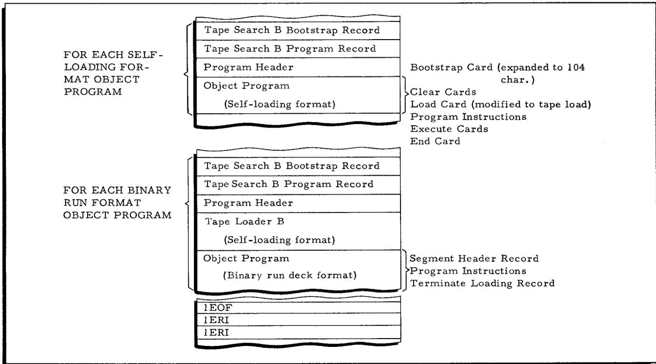
Figure C-2. Self-loading Tape (SLT) Format
