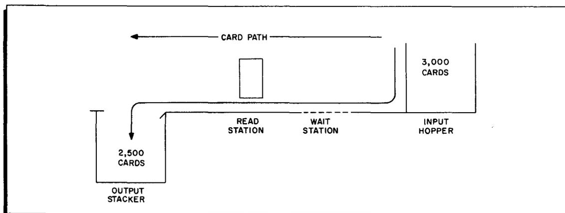
Figure 3-1. Card Path in Type 123 Card Reader
