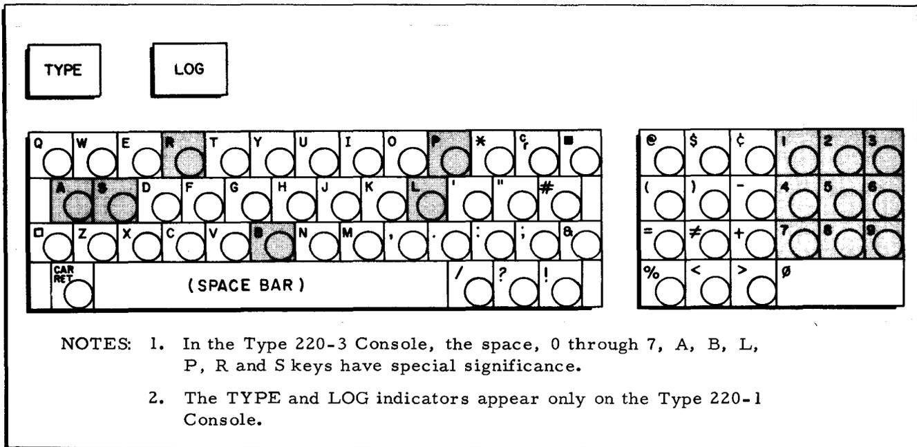
Figure 8-2. Console Keyboard Layout
