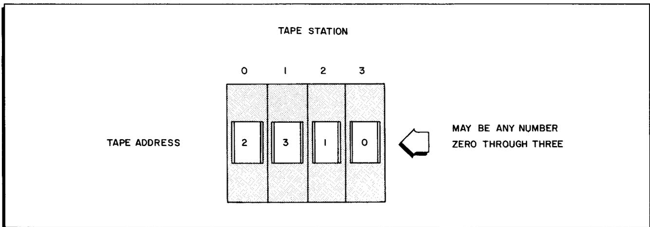
Figure 7-1. Manual Controls for Type 103 Tape Control
