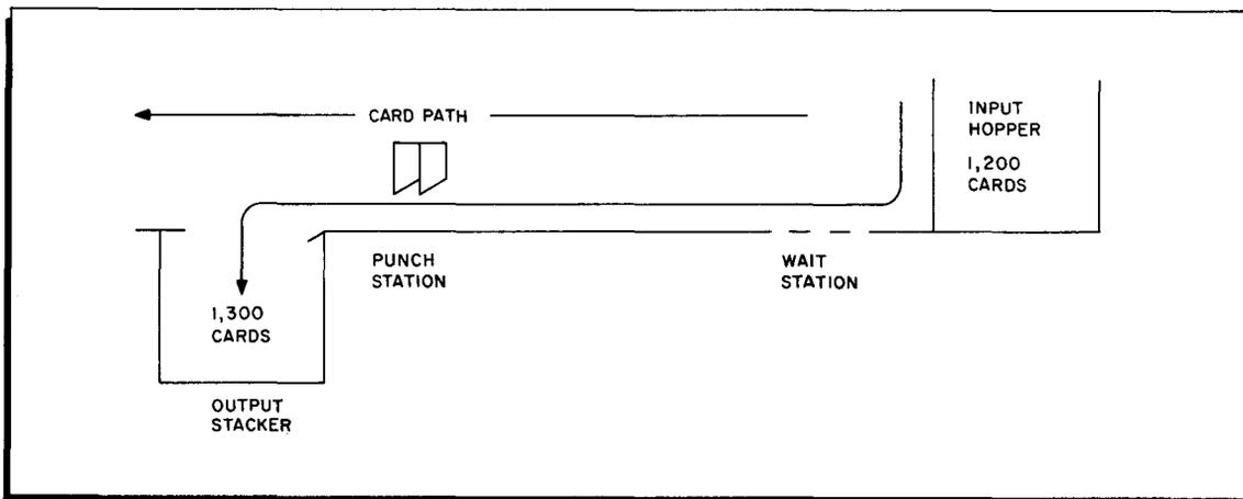
Figure 4-1. Card Path in Type 214-1 Card Punch
