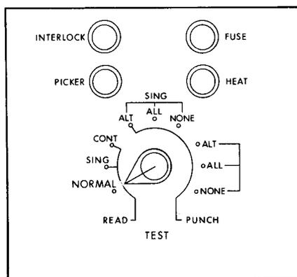
Figure 4-2. Auxiliary Control Panel Controls and Indicators
