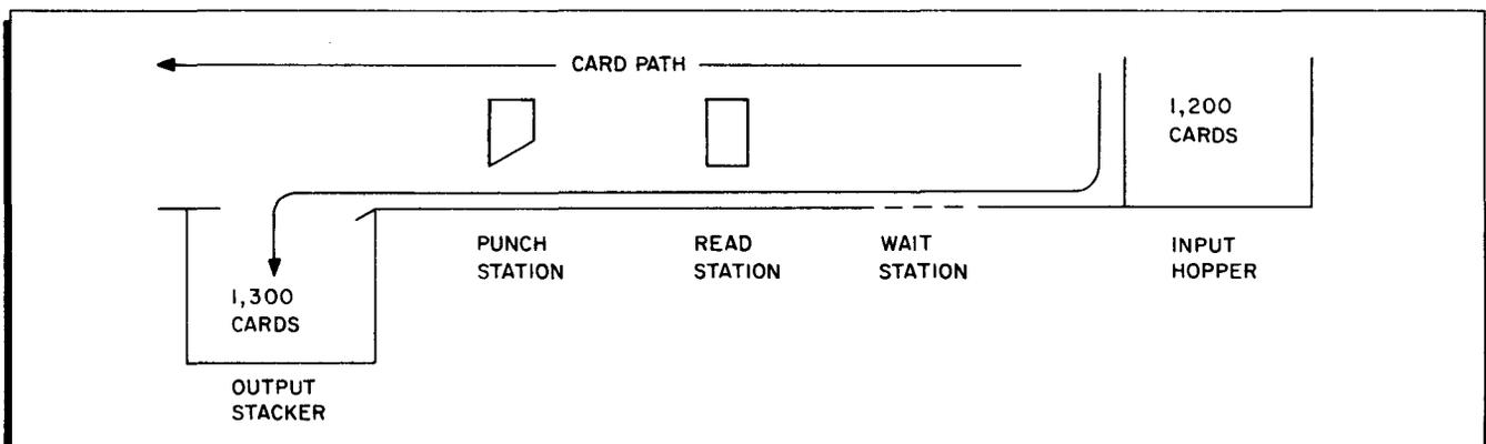
Figure 5-1. Card Path in Type 214-2 Card Reader/Punch
