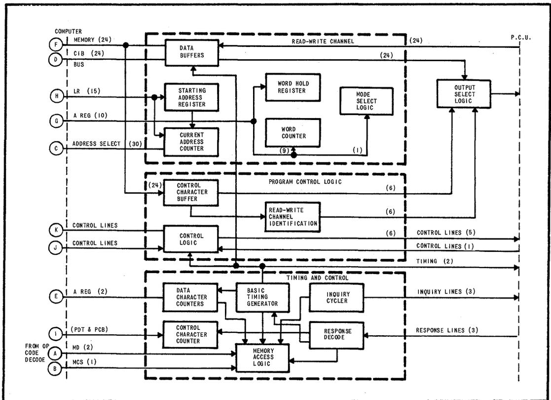
FIGURE 9. THE BUFFERED INPUT/OUTPUT CHANNEL.
