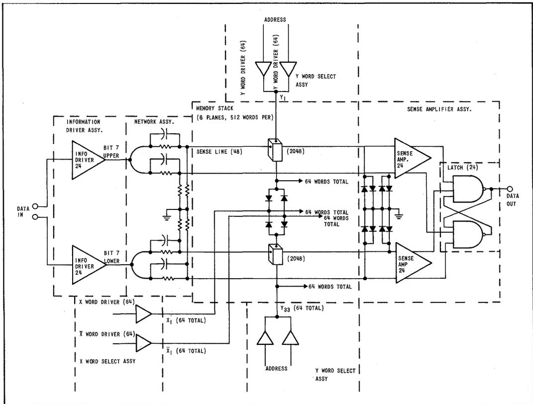
FIGURE 16. READ, WRITE, AND SELECTION SCHEME.
