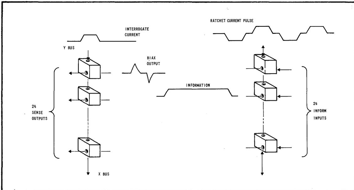
FIGURE 11. READ AND WRITE SIGNALS FOR BIAX ELEMENTS.
