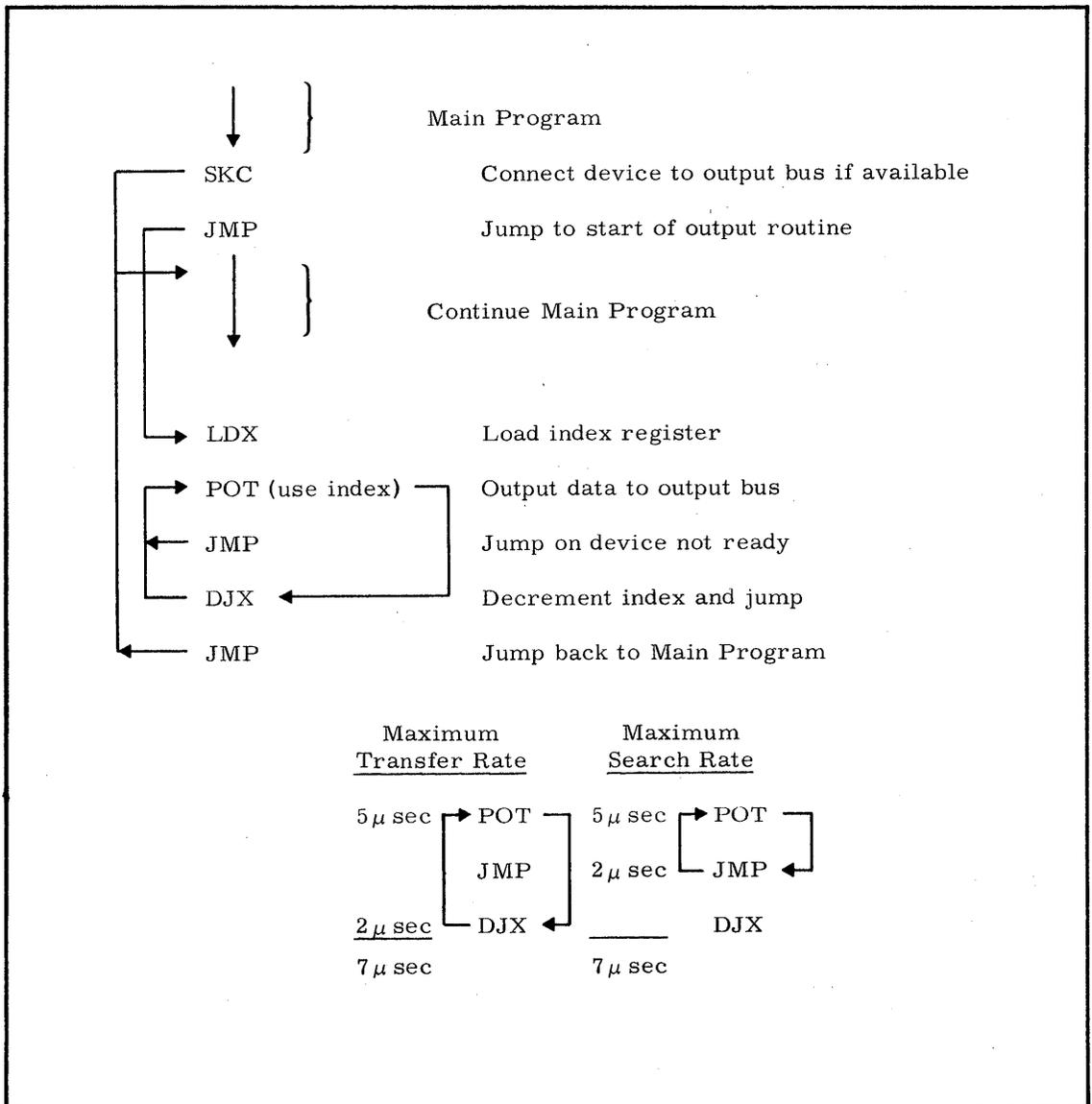
FIGURE 7. PROCEDURE AND RATE FOR MAXIMUM OUTPUT TRANSFER.
