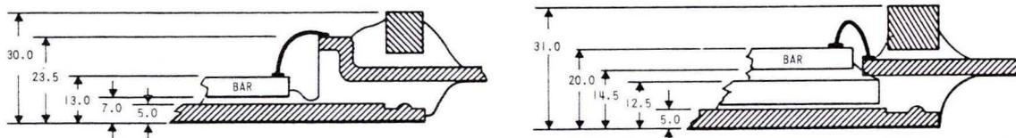
FIGURE 21. BARE BASE RAISED LEAD HEADER (LEFT); PRESENT APPROVED HEADER (RIGHT).
