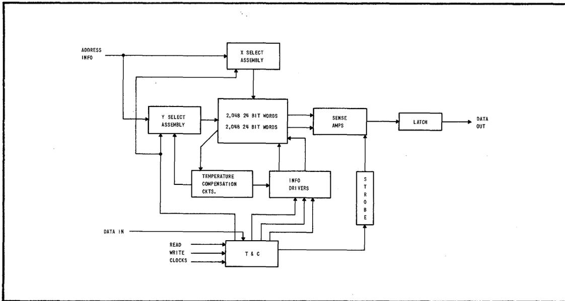
FIGURE 15. THE MEMORY STACK AND ASSOCIATED ELECTRONICS.
