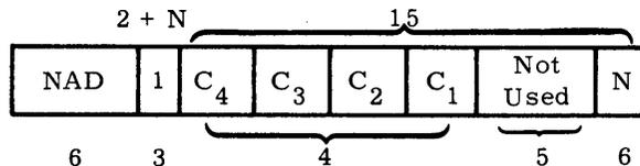
Shift (A), or, in the case of double-precision, shift the contents of A and B taken together as a 48-bit register, by N bits, as follows:
