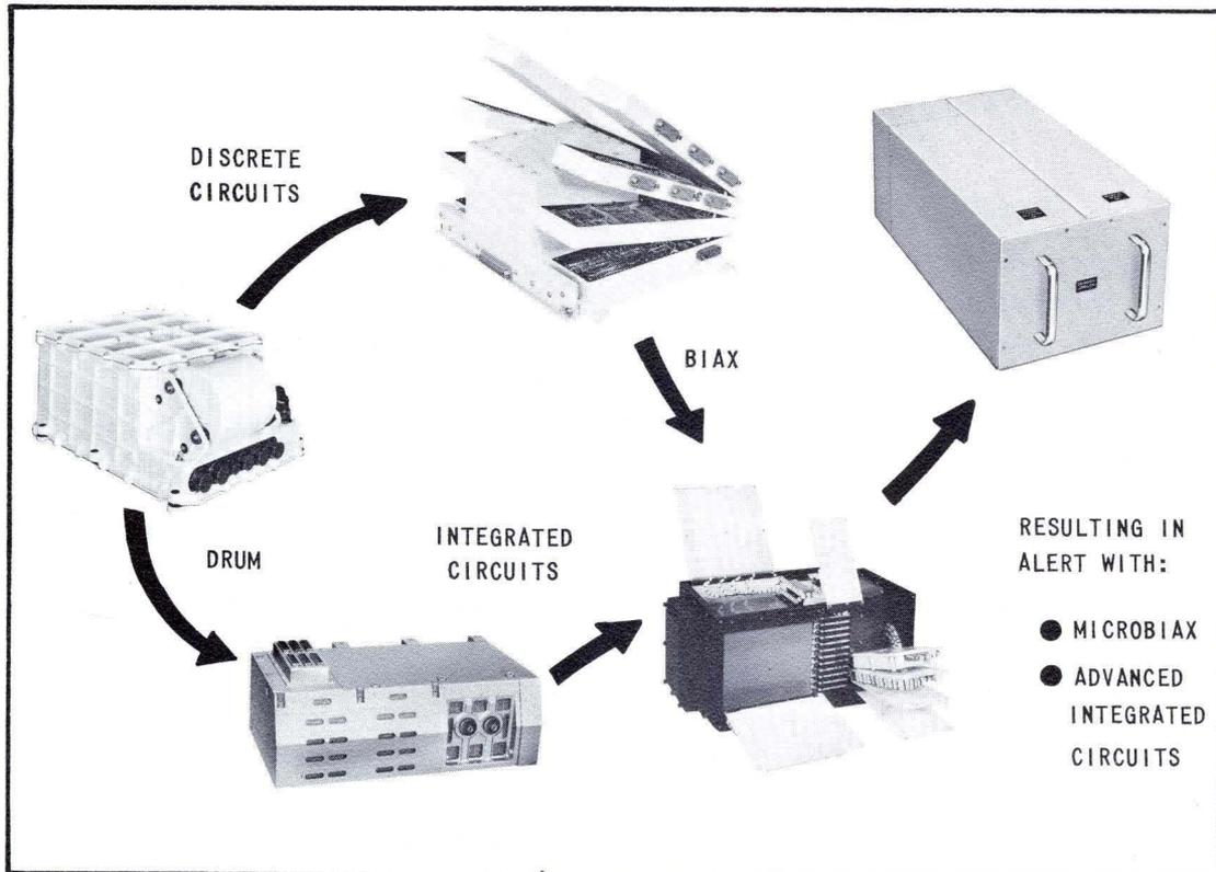
FIGURE 1. COMBINATIONS OF CIRCUITRY AND MEMORIES LEADING TO ALERT.
