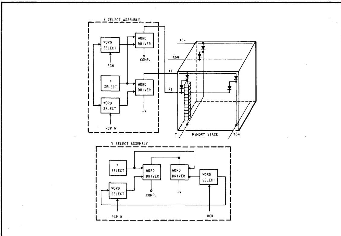
FIGURE 13. THE SELECTION MATRIX SHOWING X AND Y SELECT ASSEMBLIES.
