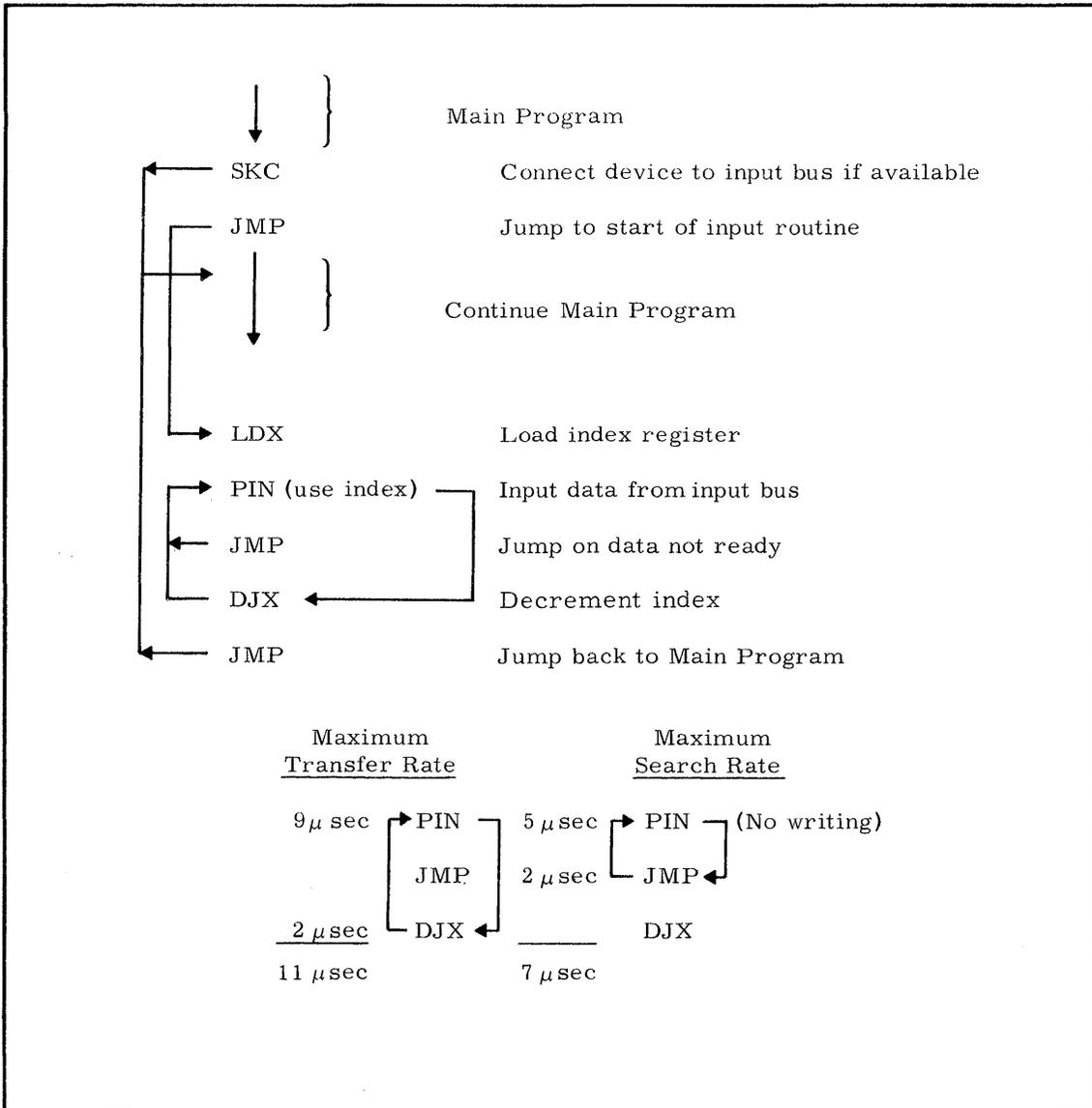
FIGURE 6. PROCEDURE AND RATE FOR MAXIMUM INPUT TRANSFER.
