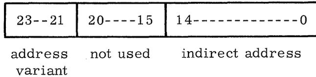
Data words are in two forms, either binary or alphanumeric. The binary word contains 23 information bits plus sign. This word is broken into segments to represent the alphanumeric word.
