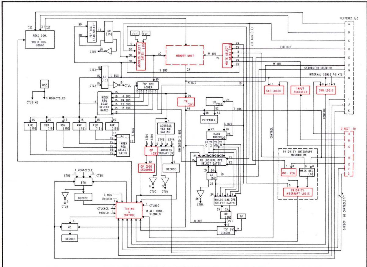
FIGURE 5. DIRECT INPUT/OUTPUT SCHEME IN CENTRAL PROCESSOR.
