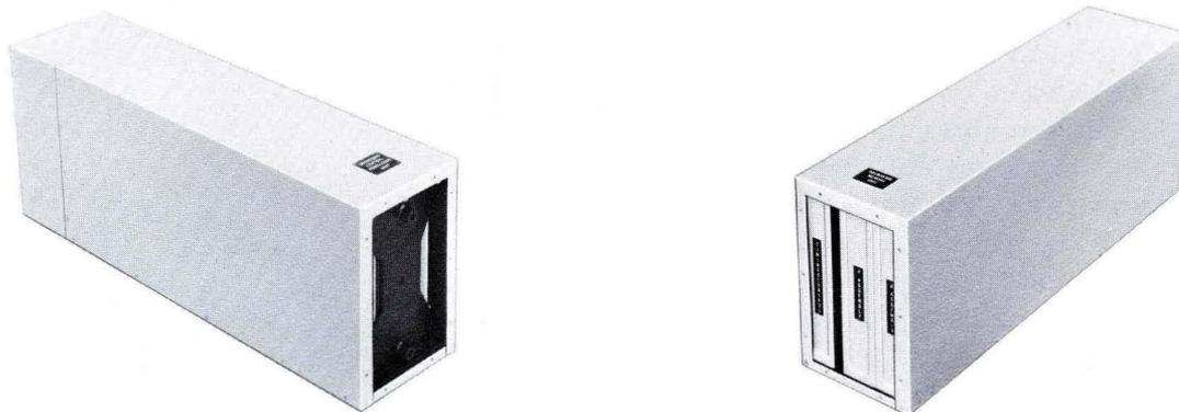
FIGURE 22. MODULAR UNITS SHOWING CENTRAL PROCESSOR (LEFT); MEMORY (RIGHT).
