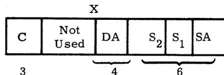
Transfer the register designated by SA to the register designated by DA, or exchange SA and DA.
