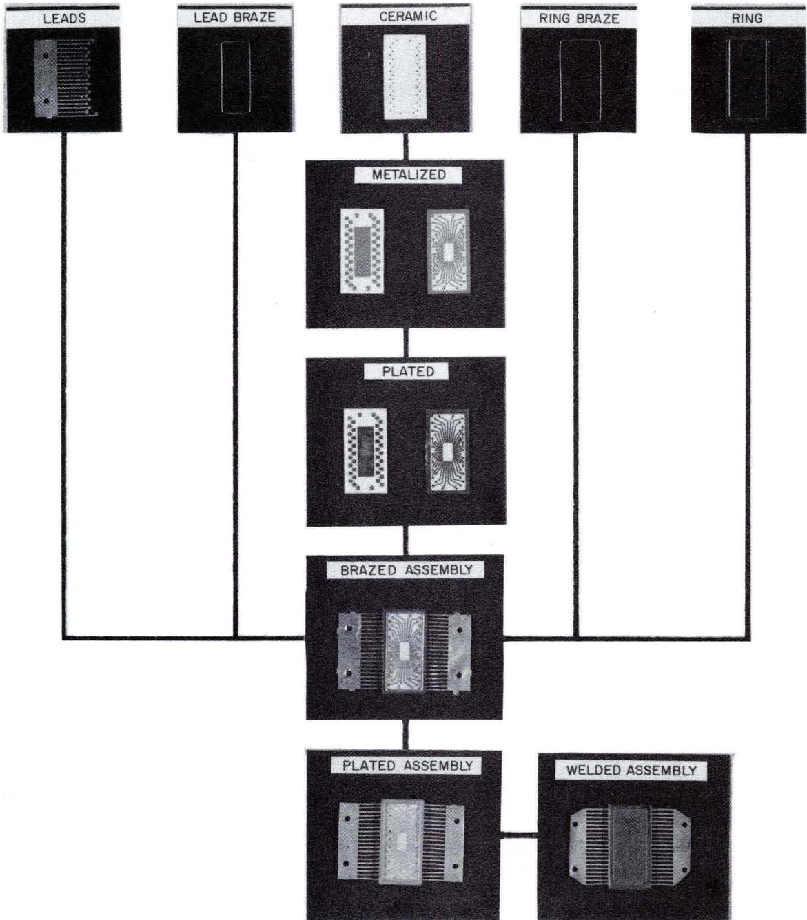
FIGURE 18. STEPS IN FLATPACK CONSTRUCTION.
