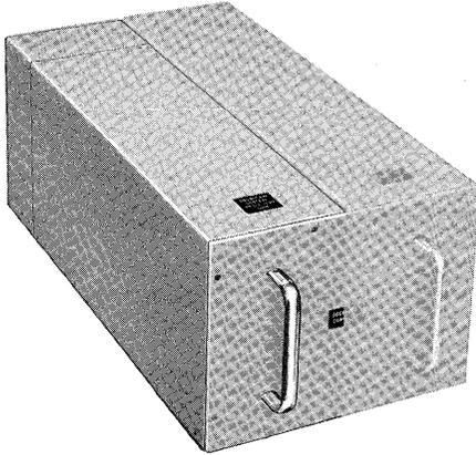
*ALERT* central processor is 5 inches by 7.6 inches by 19.5 inches and contains a direct input/output channel in addition to circuitry necessary to perform arithmetic functions. Characteristics include:
