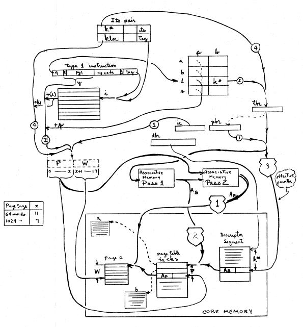
We show two primary routes to the block address of page c of segment <k>. Route l is through the 2-stage associative memory mechanism. Route 3 is through the descriptor segment mechanism. Route 2 is an intermediate route; i.e., via the lstage associative memory to the page table for segment <k>.
