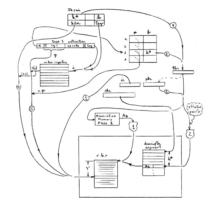
This shows two routes to the block address of segment < k >. Route 1 through associative memory (Figure 1-22), and Route 2 through the descriptor segment mechanism.
