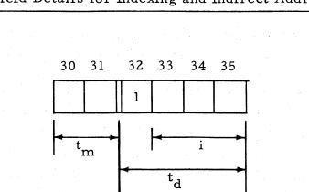
TABLE 1-2 Tag Field Details for Indexing and Indirect Addressing
