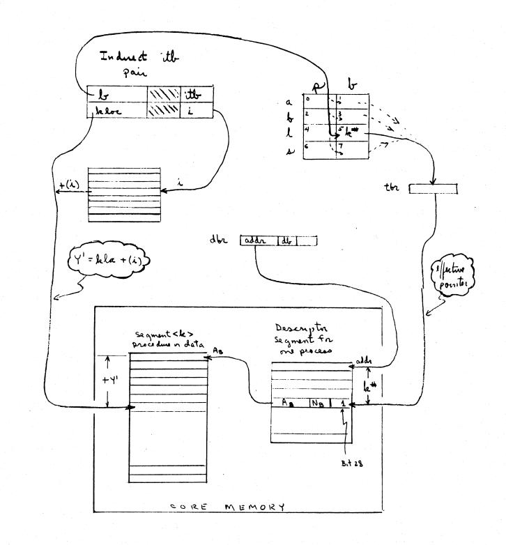
Figure 1-17. Address Formation for itb Pairs
