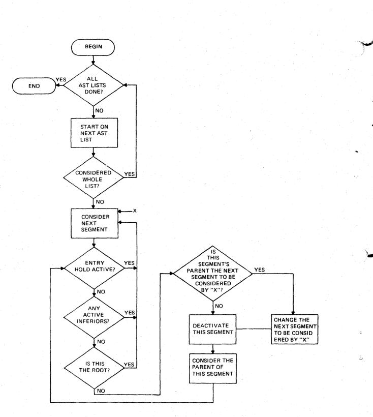
Figure 4-2. Deactivation Loop of Shutdown
