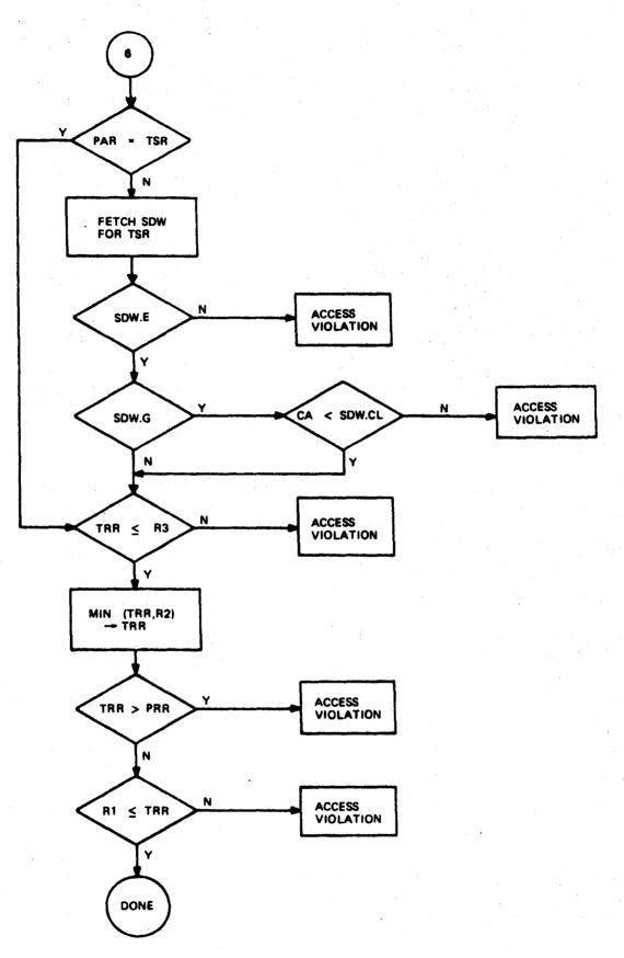
Figure 6. Access Checks for CALL Instruction
