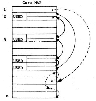
The n<sup>th</sup> CME refers to n<sup>th</sup> 1024-word block of core. Figure 3. The System Segment Table
