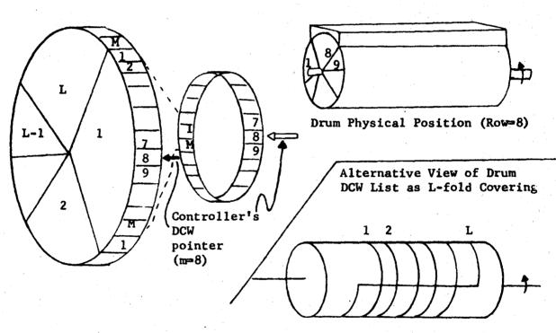
Figure 2. Drum DCW List Configuration
