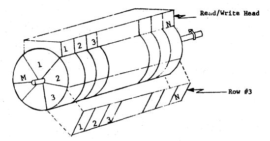
Figure 1. Drum Configuration
