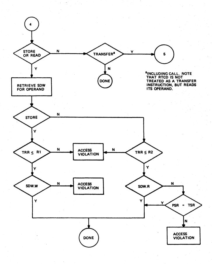
Figure 4. Access Checks for Nontransfer Instructions
