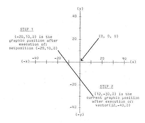
Figure 2-1. Current Graphic Position Modification
