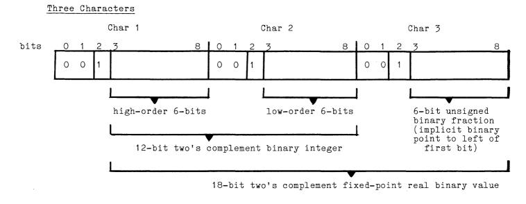
Figure 3-5. Scaled Fixed-Point Format
