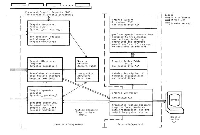
Figure 3-1. Functional Parts of the Multics Graphics System
