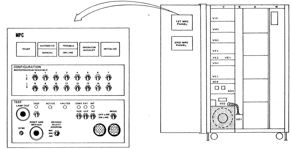
(WCPU66LA) CPU CABINET LEFT DOOR OPEN, RIGHT DOOR REMOVED
