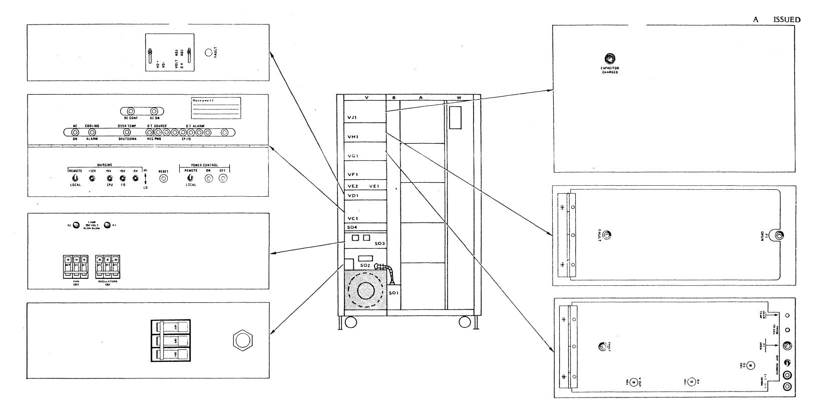
FIGURE 2-10 MPC POWER PANELS
