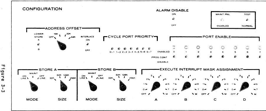
System Controller Configuration Panel
