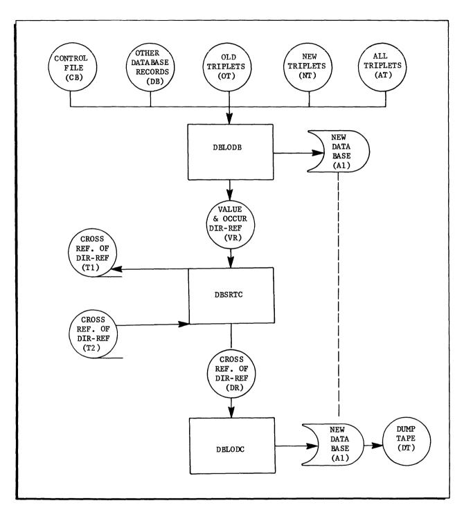
Figure 1-5. Phase IV - File Load Block Diagram
