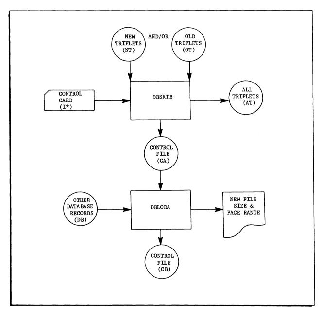
Figure 1-4. Phase III - File Merge Block Diagram
