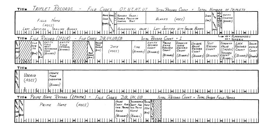
Figure C-1. dataBASIC Load/Unload System Tape Formats
