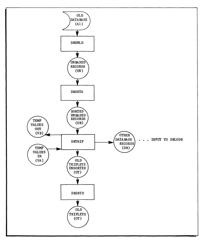
Figure 1-3. Phase II - File Unload Block Diagram
