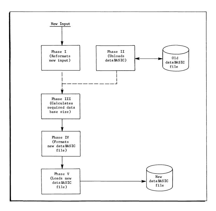
Figure 1-1. dataBASIC Load/Unload System Flow
