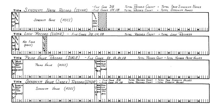
Figure C-1. dataBASIC Load/Unload System Tape Formats (continued)
