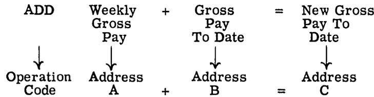
Here the first 3 letters indicate the operation (ADD), the next 4 digits specify the address (Address A) or location in the 2000 word memory containing the Weekly Gross Pay, the next 4 digits (Address B) specify the address of the Gross Pay to Date and the last 4 digits (Address C) specify the location where the result of the addition (New Gross Pay to Date) shall be stored.
