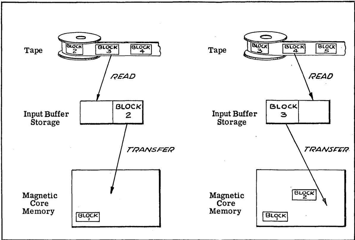
Figure 6. Input Buffer Storage.
