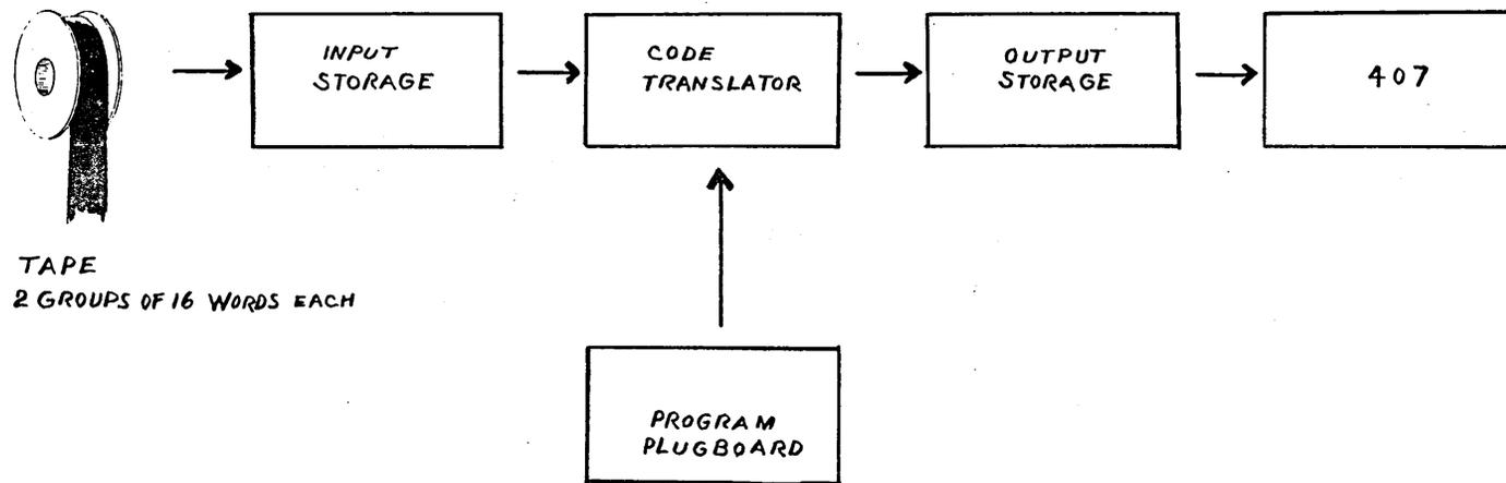
Figure 16. DATAmatic Output Converter Type 1300 Block Diagram.
