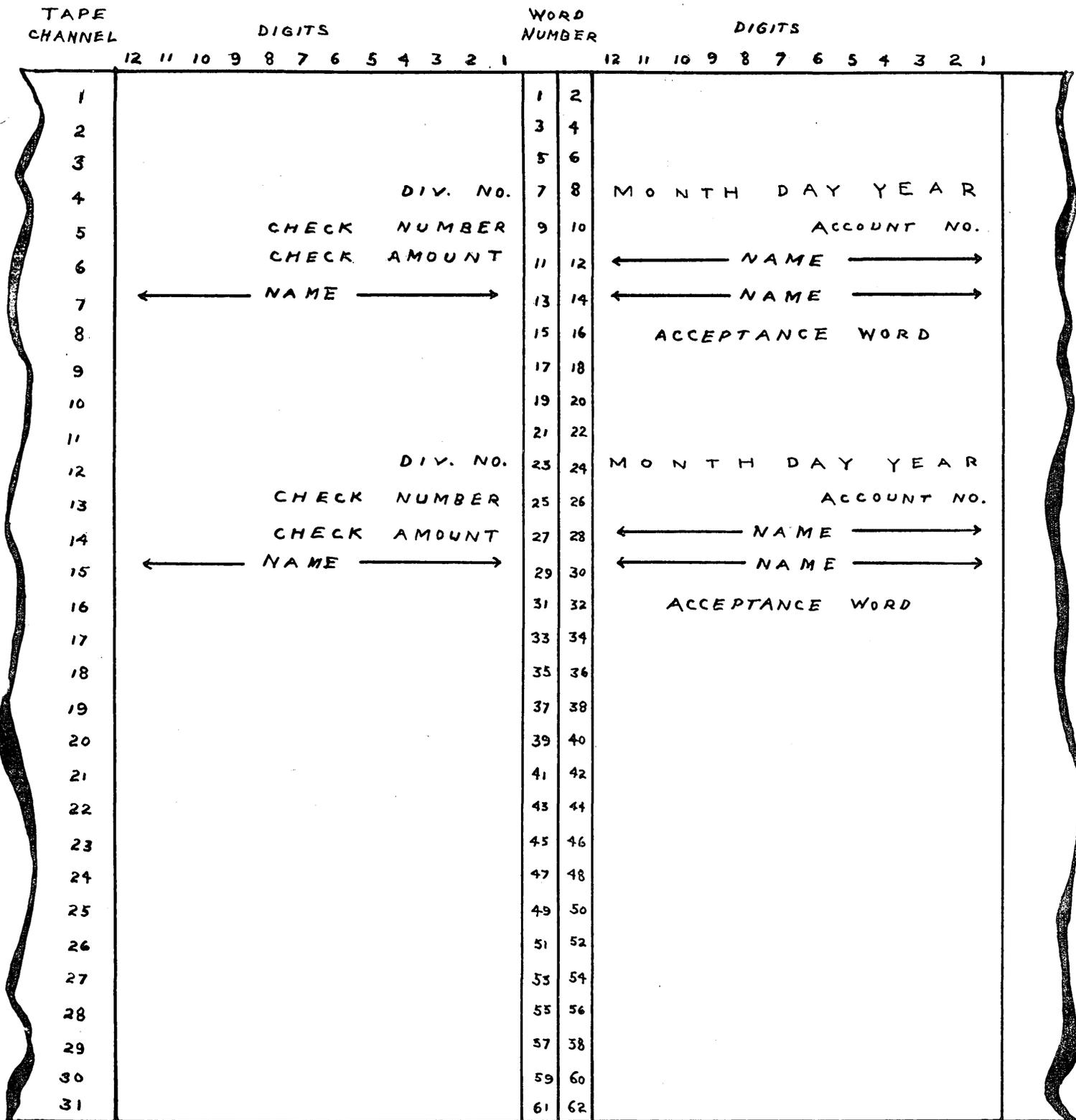
Figure 18. Tape Format for Typical Dividend Checks.
