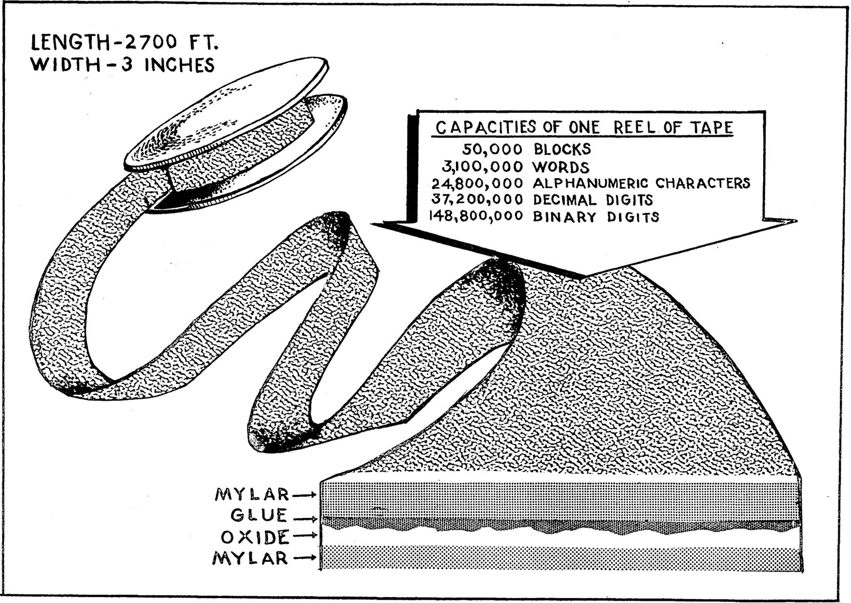
Figure 1. DATAmatic 1000 Magnetic Tape .
