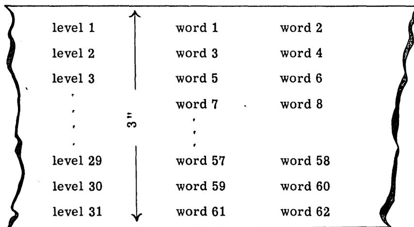
Figure 2. Arrangement of Words on Magnetic Tape.
