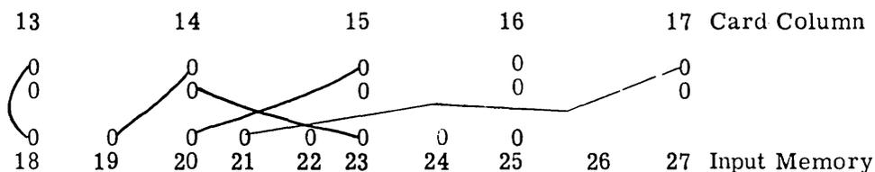
In this diagram, card column 13 is wired to position 18, card column 14 to positions 19 and 23, column 15 to positions 20 and 22, column 16 discarded and column 17 wired to position 21. It should be noted that all transposition, duplication, and discarding of information from the card must be done with this plugboard which is called the Card Reader Plugboard.
