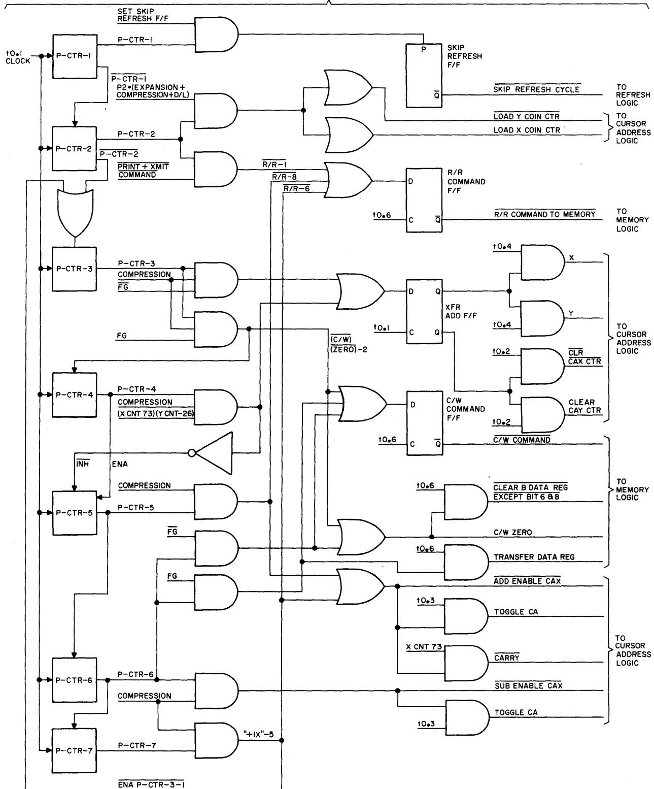
Figure 3-40. DELETE CHARACTER Logic Flow Diagram
