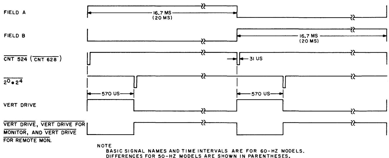
Figure 3-8. Vertical Drive Generator, Timing Diagram
