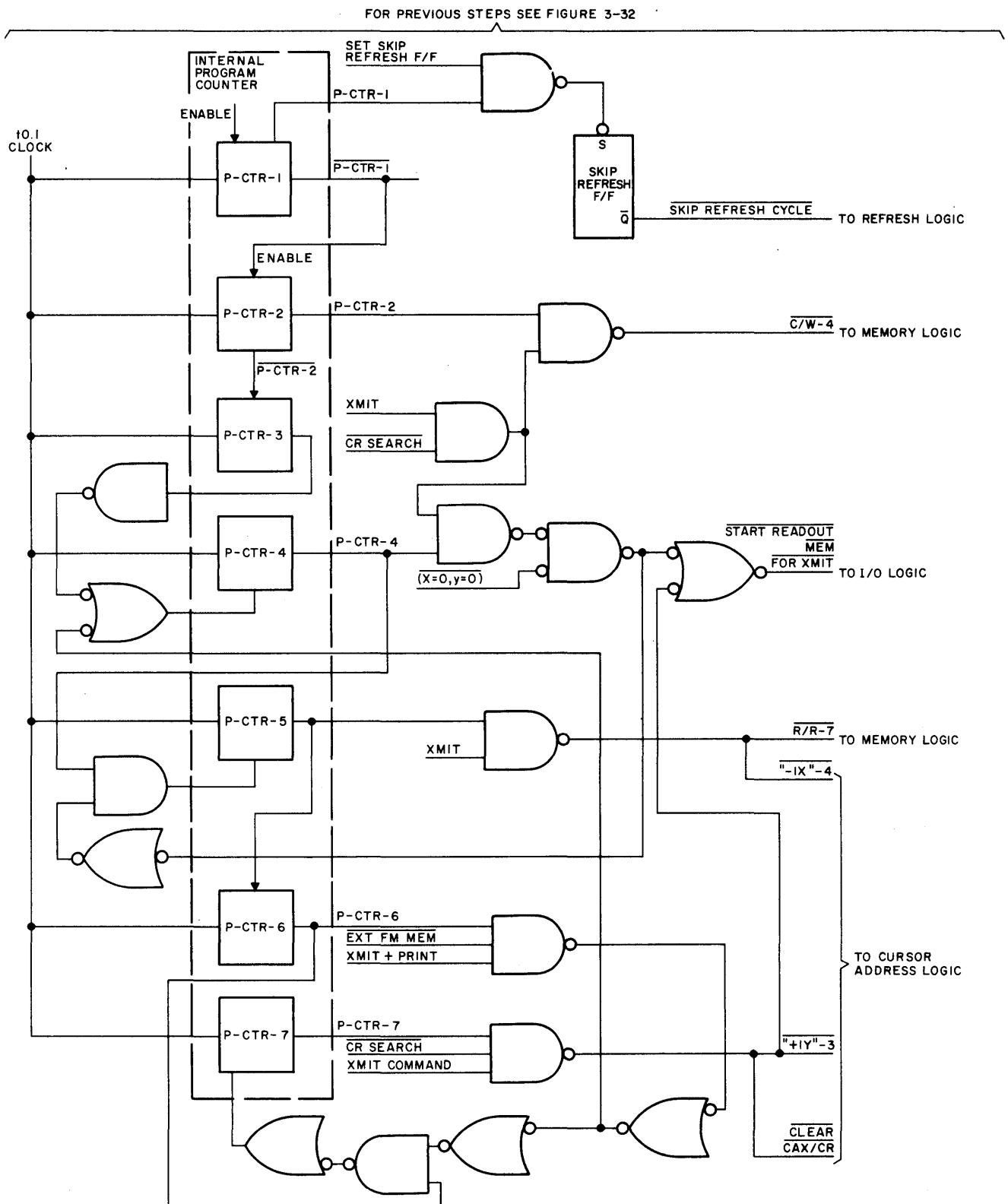
Figure 3-41. TRANSMIT Logic Flow Diagram
