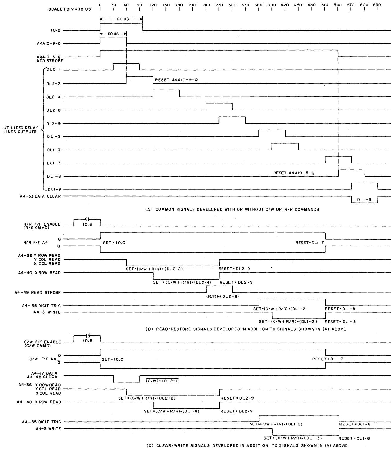
Figure 3-15. Memory Control Timing Diagram
