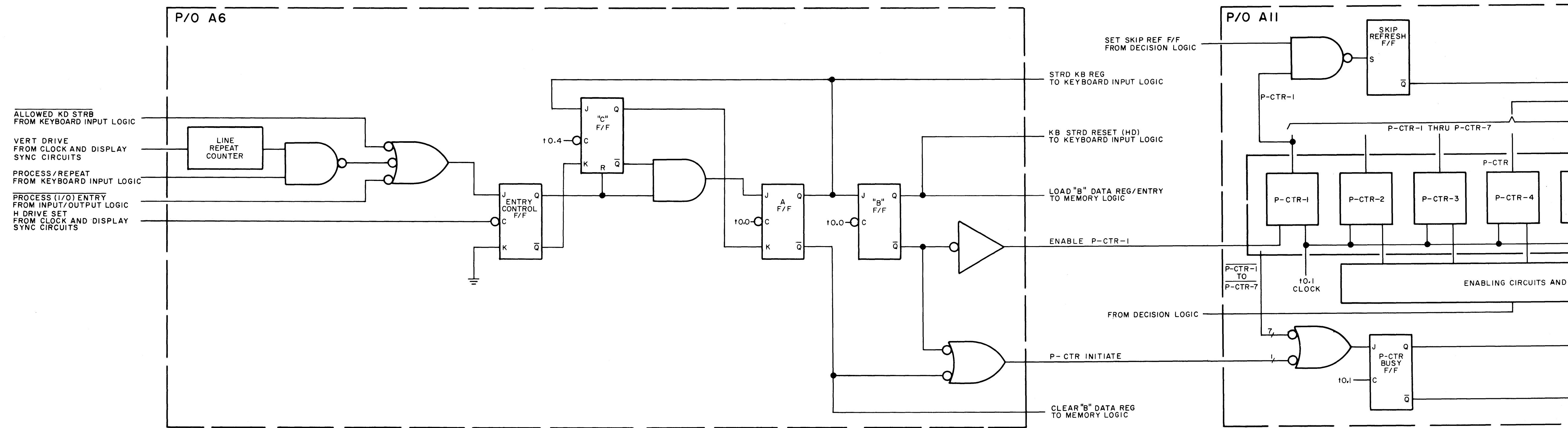
Figure 3-12. Internal Program Counter Block Diagram
