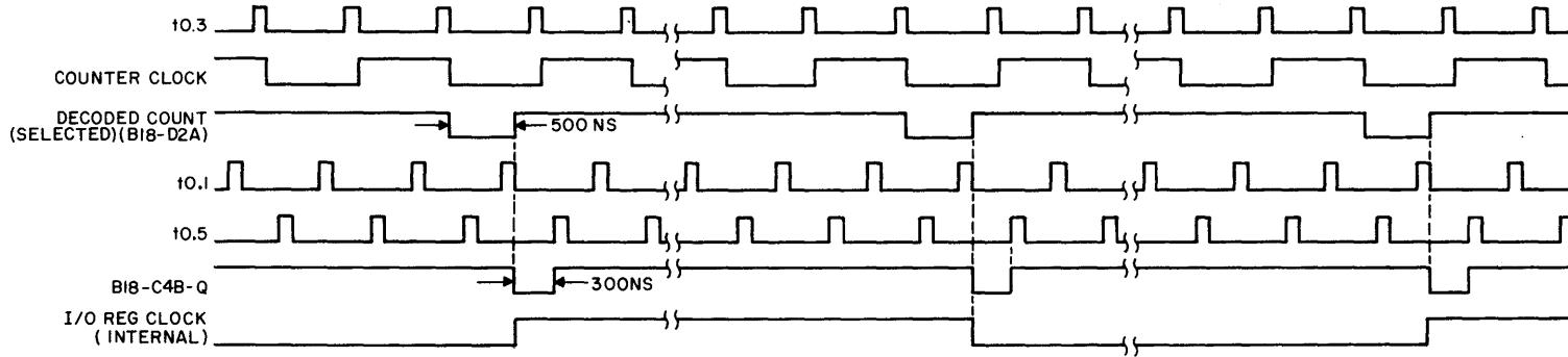
Figure 3-17. I/O Register Clock, Logic Diagram
