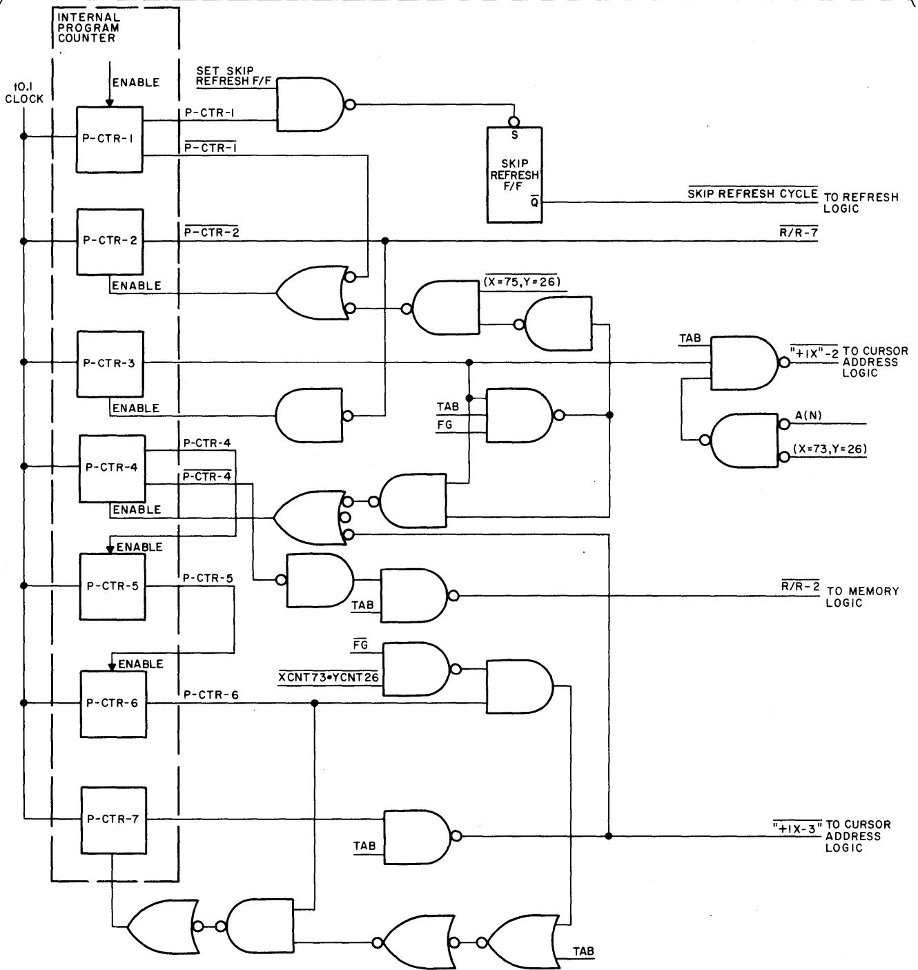
Figure 3-42. TAB Logic Flow Diagram
