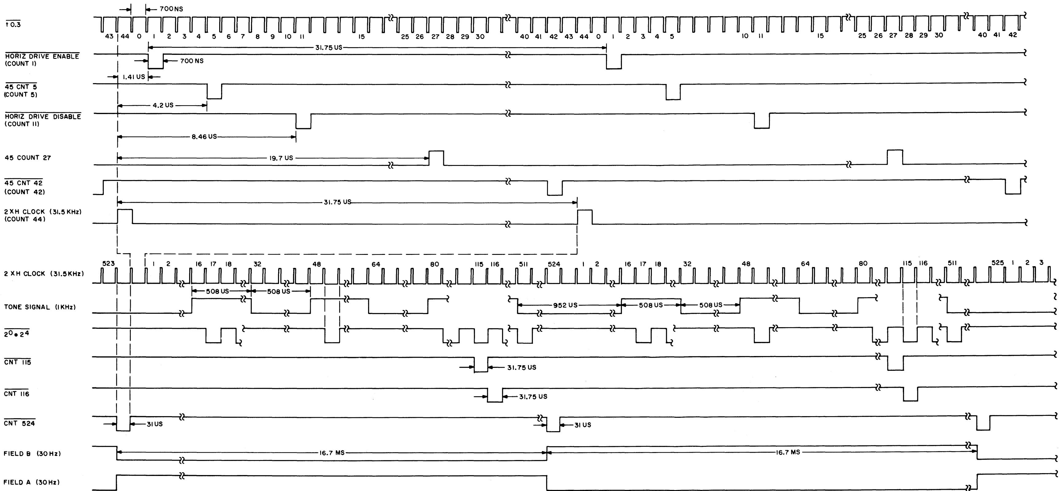
Figure 3-6. Divide by 45 and Divide by 525 Counters (50-Hz Models), Timing Diagram
