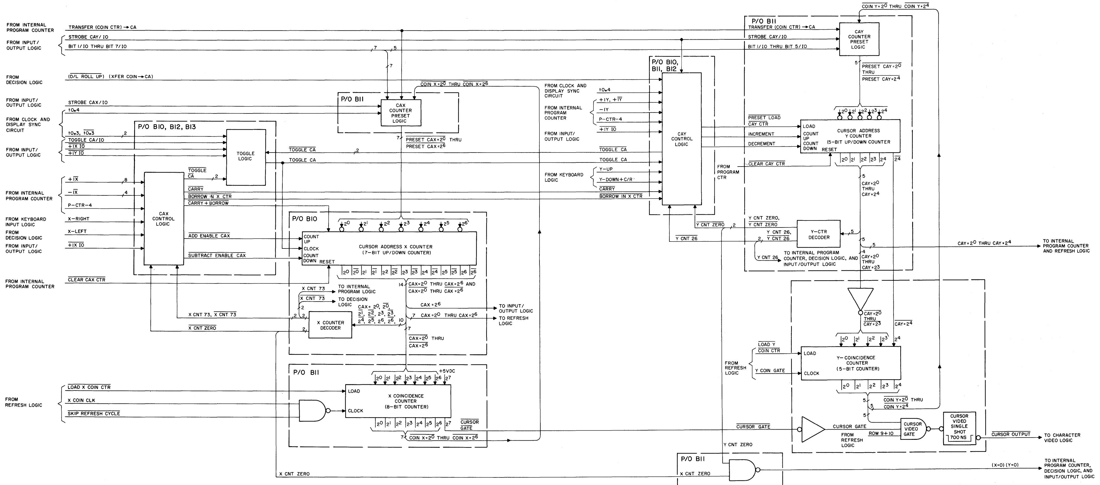
Figure 3-26. Cursor Address Logic, Functional Block Diagram
