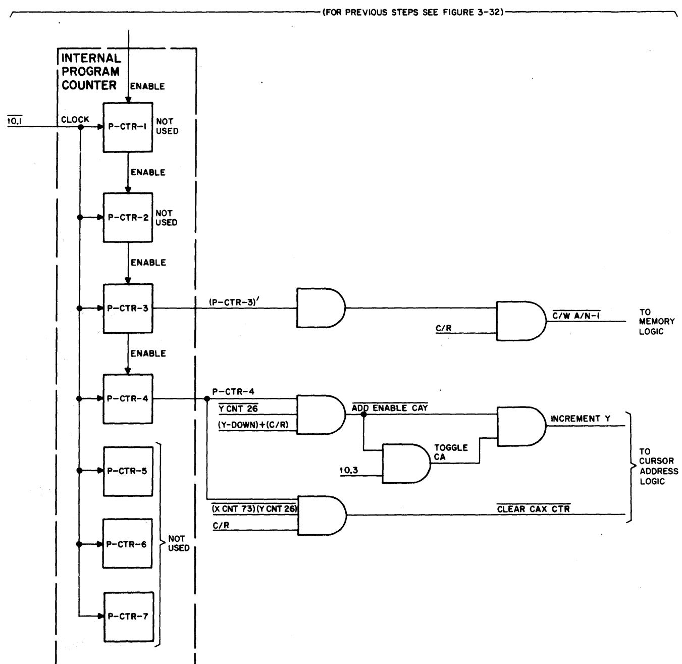
Figure 3-33. C/R Logic Flow Diagram
