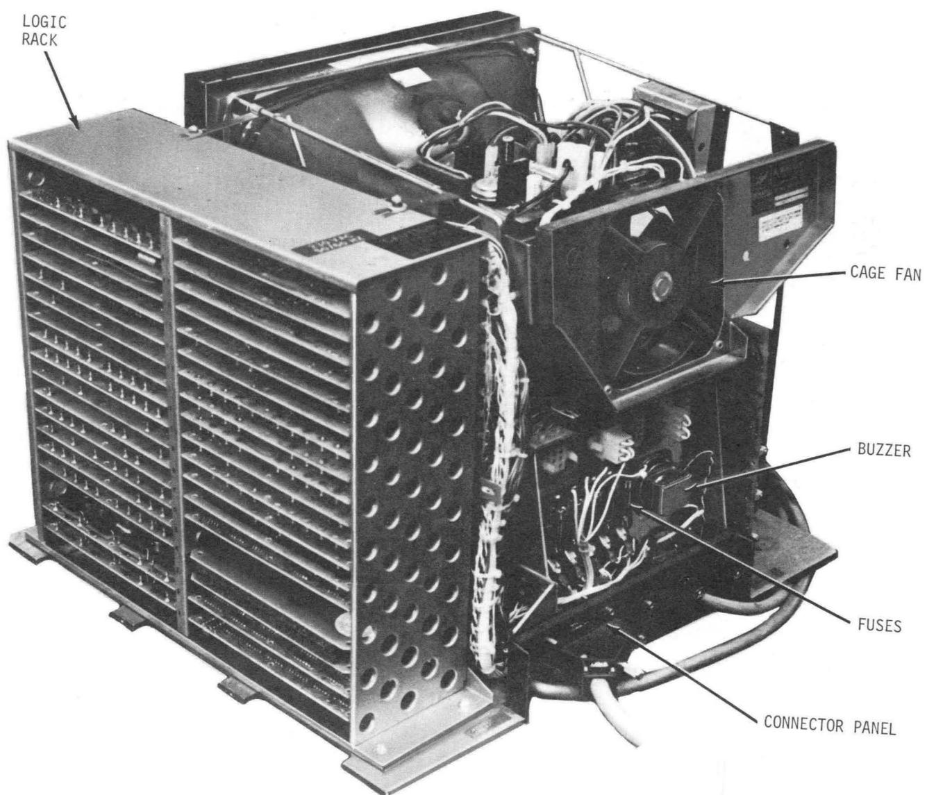
Figure 2-3. Display Unit, Rear Right Side View
