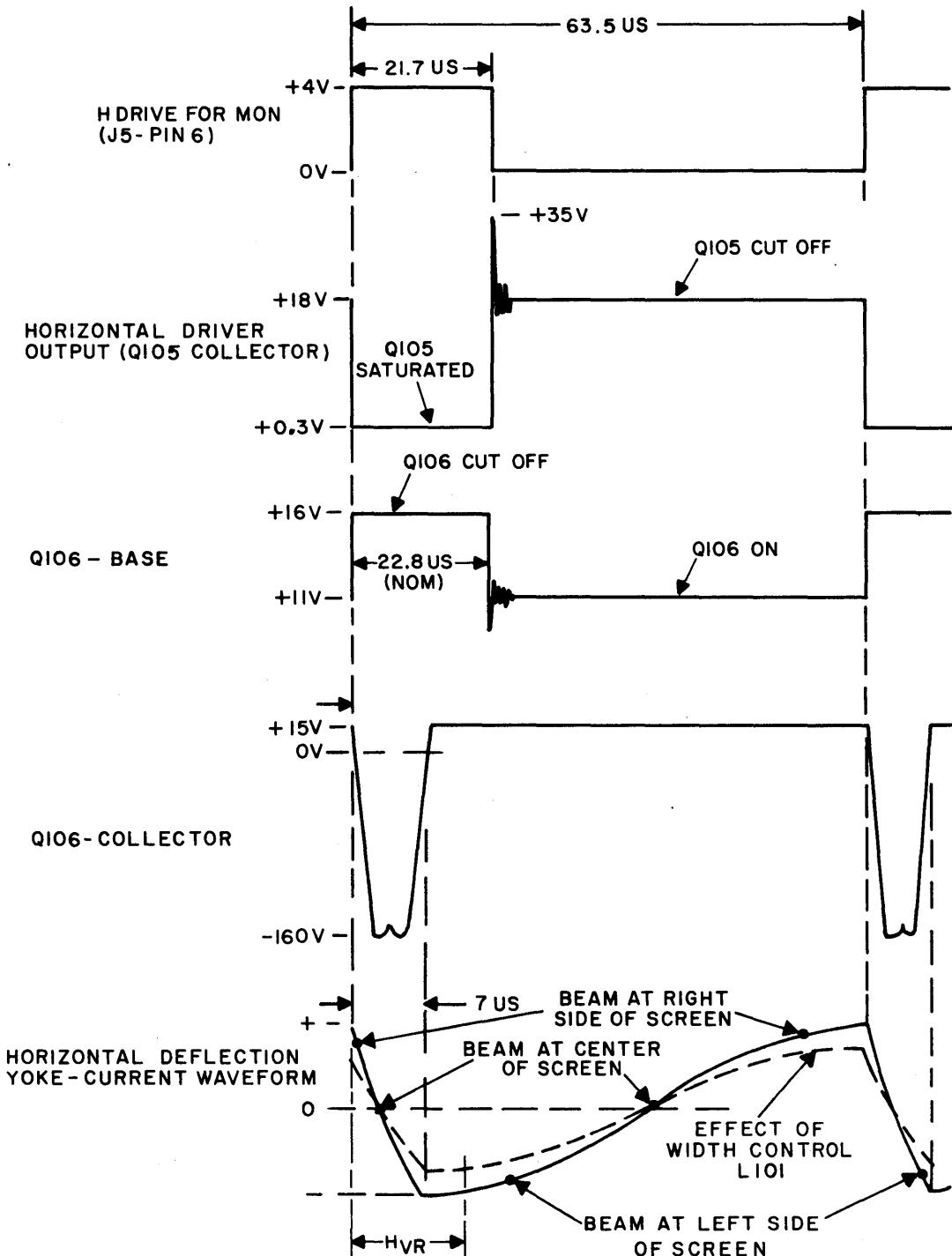
$H_{VR} = \text{TOTAL RETRACE TIME} = 9.5 \mu\text{s} (\text{INCLUDES DEFLECTION DELAY TIME})$
