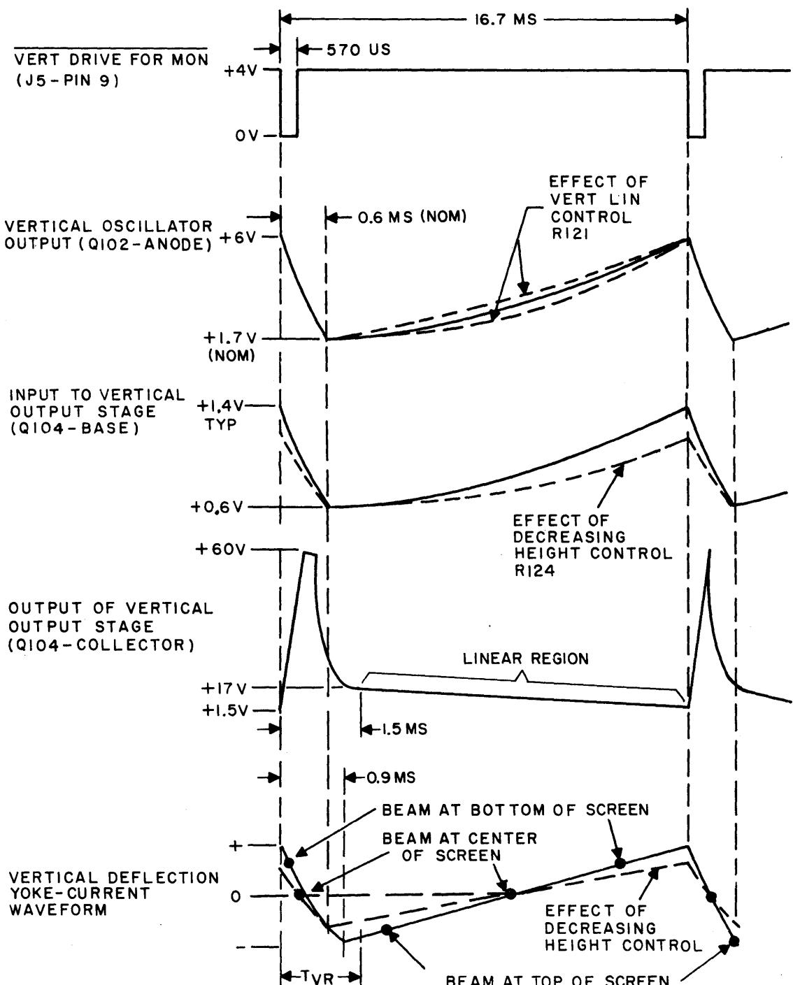
$T_{VR} = \text{TOTAL RETRACE TIME} = 1.2 \text{ MS} (\text{INCLUDES DEFLECTION DELAY})$
