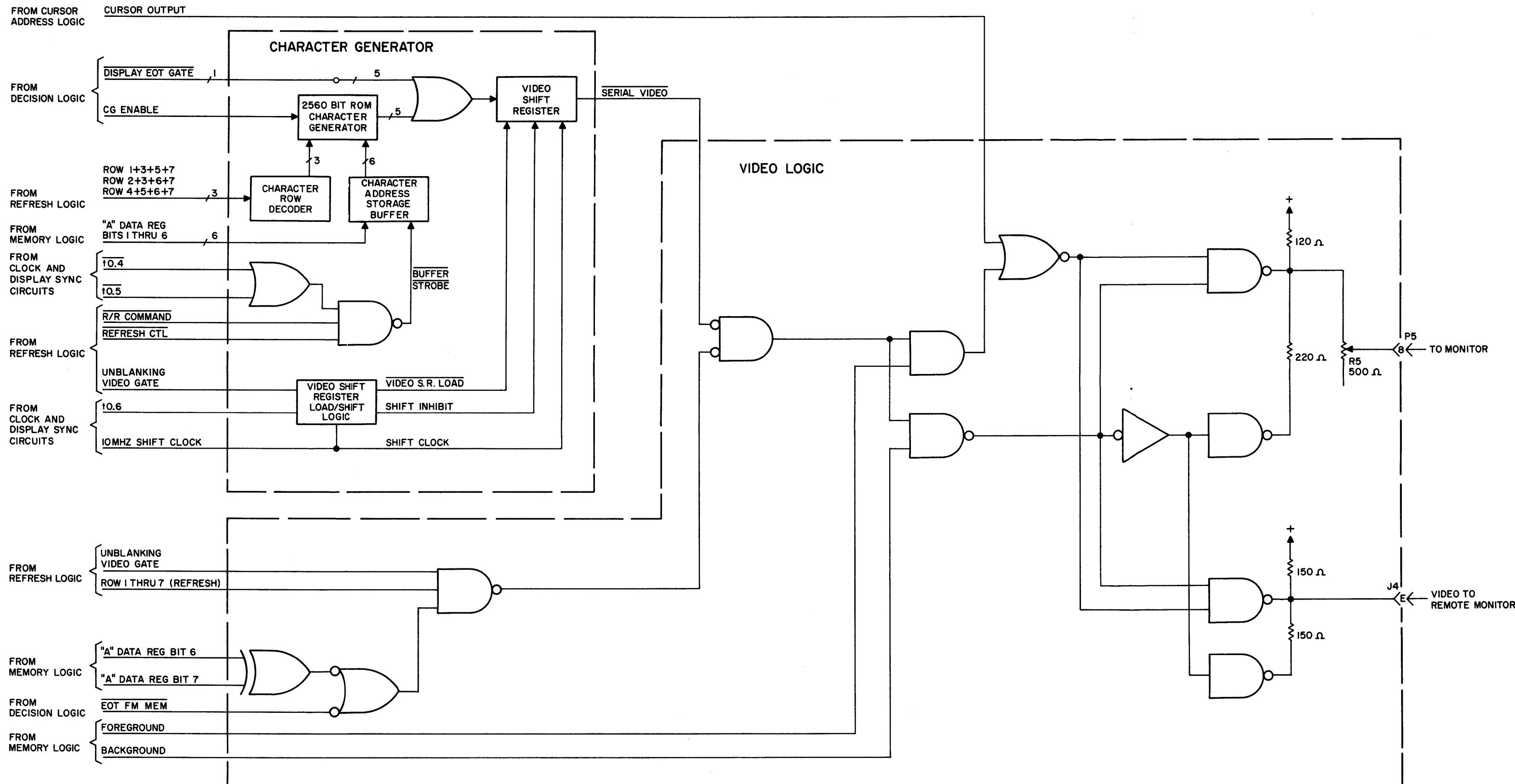
Figure 3-27. Character Video Logic Block Diagram
